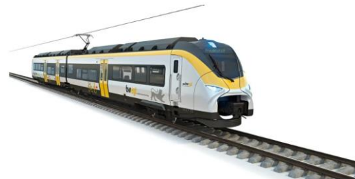
Siemens Mobility's battery powered Mireo Plus B
