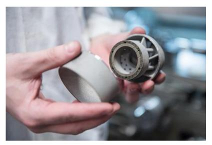
**3D-printed gas turbine burner heads for commercial power plant operation**Siemens uses Additive Manufacturing to produce various gas turbine components.
