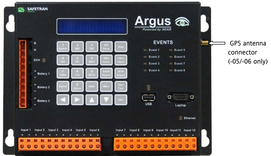
Figure 1-3. ARGUS (-02/-03 & -05/-06) Front Panel Generic Overlay
