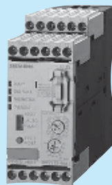
3RB22/23 overload relays up to 820 A for full motor protection, CLASS 5 to CLASS 30 adjustable
