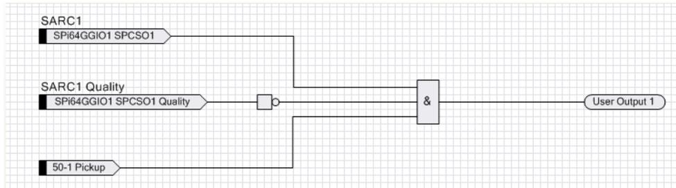
Figure 43: Relay Logic - SARC 1
