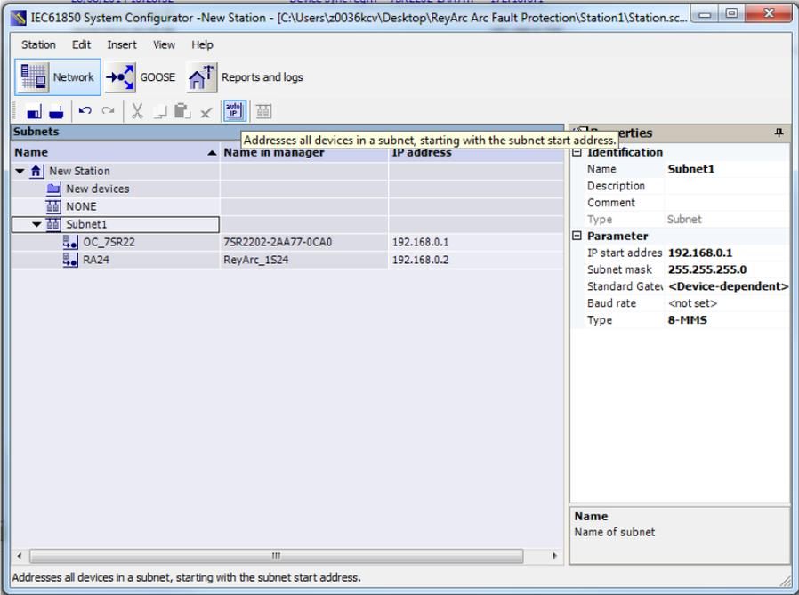
Figure 31: System Configurator - IP Address 4
