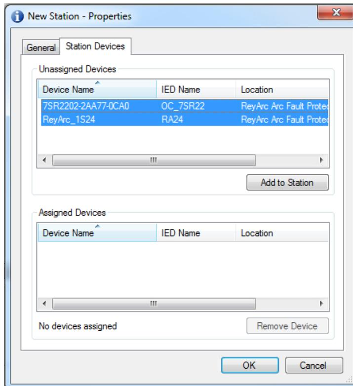
**Figure 22: Add Device to IEC61850 Station**
