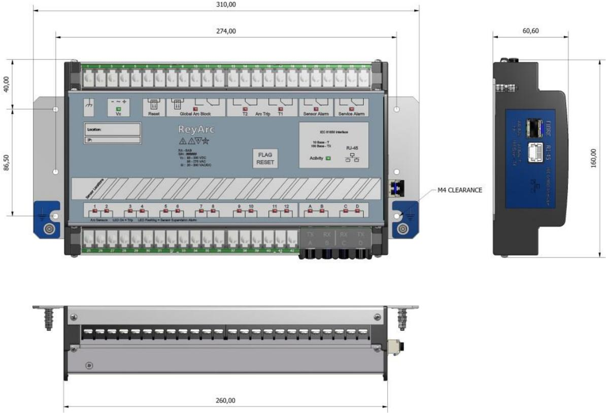
Figure 16: Terminal Layout and Module Dimensions
