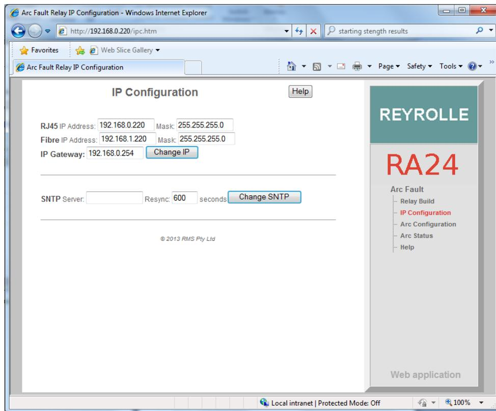
Figure 4: RA24 IP Configuration
