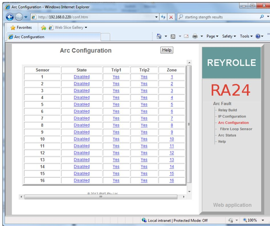
Figure 5: RA24 Arc Configuration
