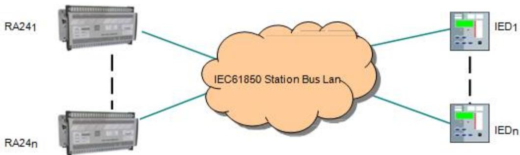
**Figure 21: RA24 IEC61850 Station LAN**
