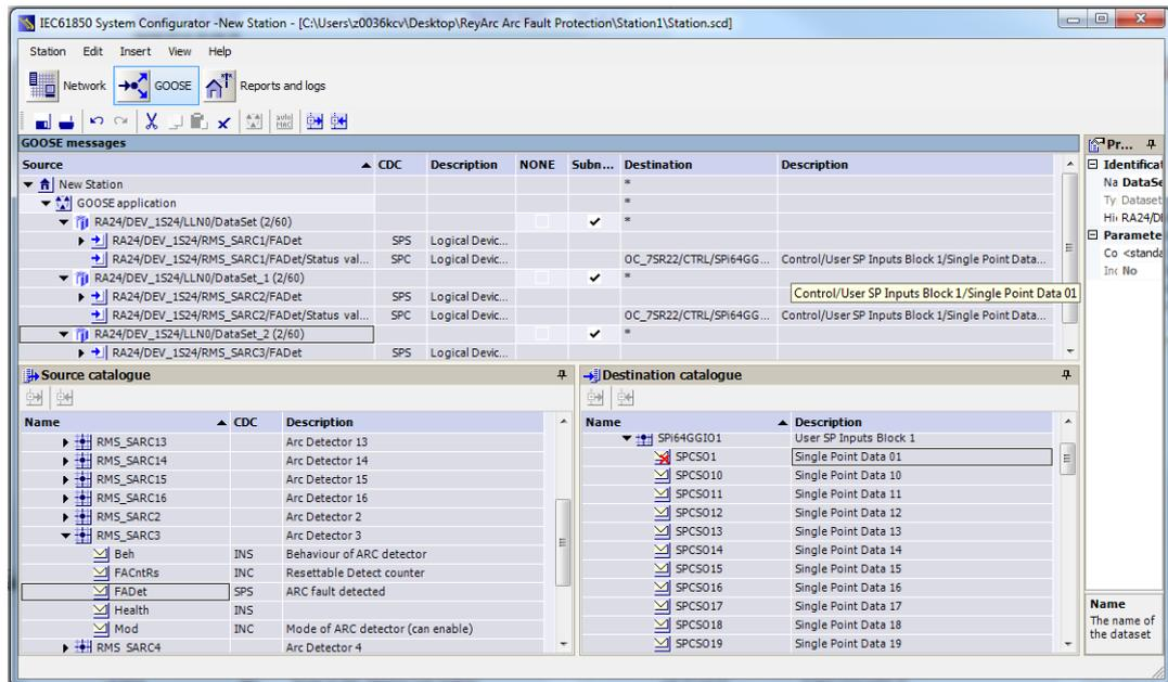
Figure 37: System Configurator - GOOSE 6
