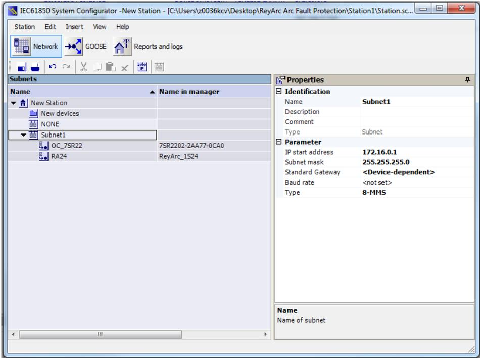
Figure 27: System Configurator - IP Address
