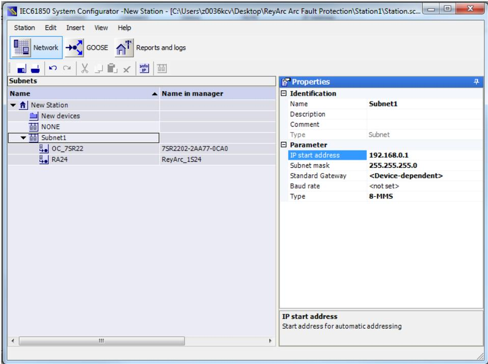
Figure 28: System Configurator - IP Address 1
