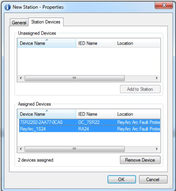
Figure 24: Add Device to IEC61850 Station 3
