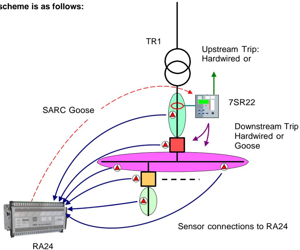
**Figure 8: RA24 Sample Protection Scheme**
