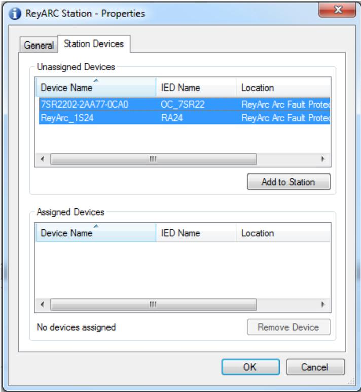
Figure 23: Add Device to IEC61850 Station 2
