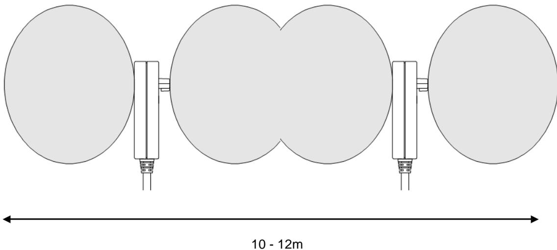
**Figure 5: RA30B Dual Detector Spacing**
