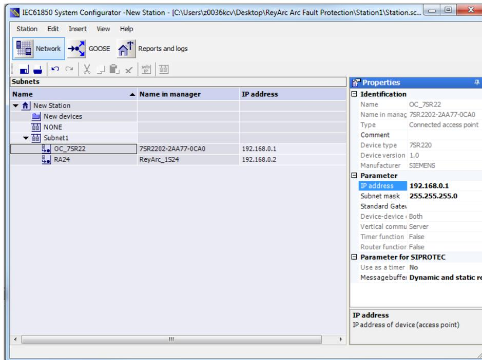
Figure 30: System Configurator - IP Address 3
