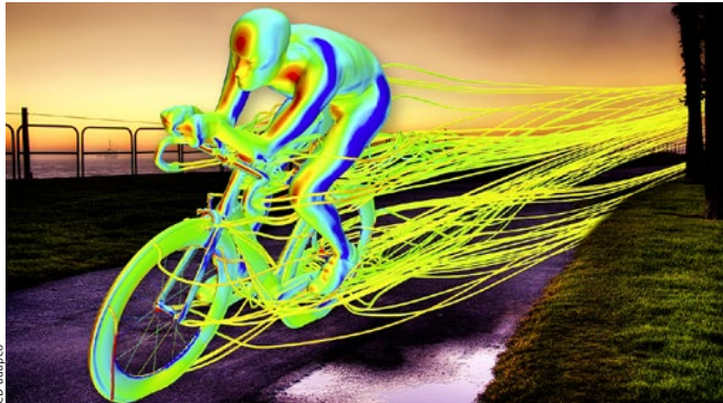
Analyzing the aerodynamics of a Cervélo bicycle
