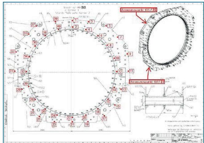
Figure 6: Test equipment; location of the 3D-vibration sensors
