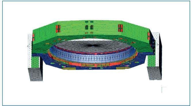
Figure 15: Finite Element Model of the Siemens 42ft GMD Ring-motor
