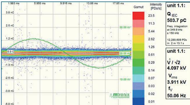
Figure 5: Partial Discharge measurement of a Siemens GMD stator coil at 4250 m a.s.l.
