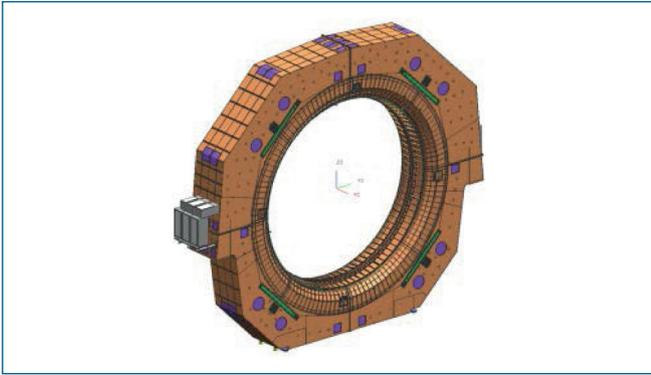
Figure 14: 3D CAD Model of the Siemens 42ft ring motor
