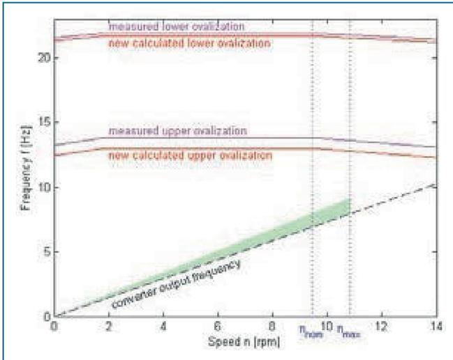
Figure 11: Campbell diagram comparing the updated FE-model with measured natural frequencies
