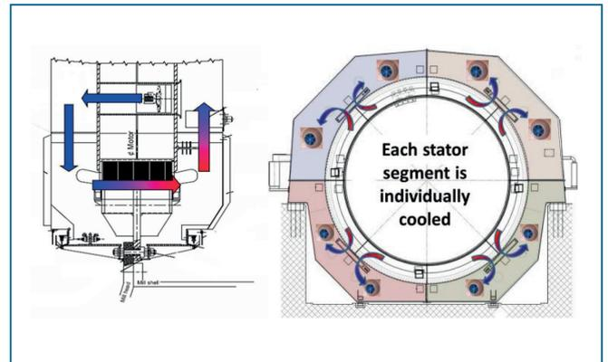
Figure 3 - Cooling scheme of the Siemens ring motor
