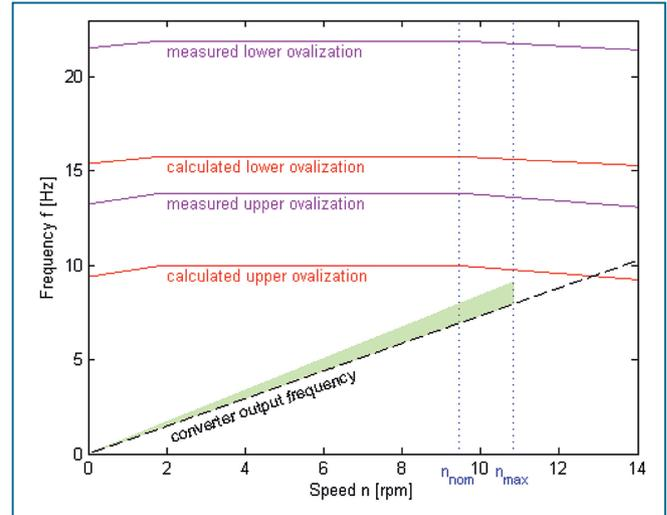
Figure 10: Campbell Diagram; comparing measured and calculated natural stator frequencies
