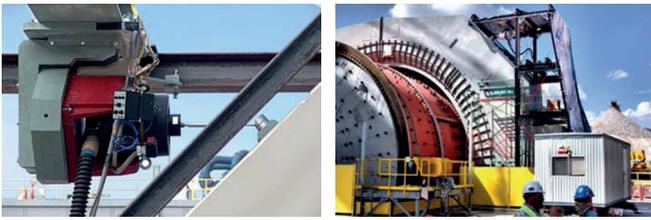
Figure 7: Vibration exciter attached to the motor housing
