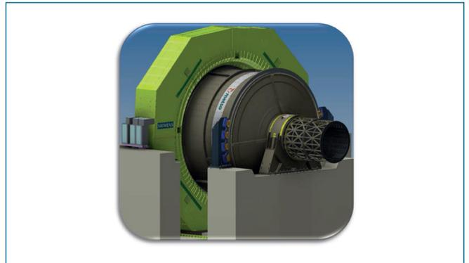
Figure 16: Computer model of a 42ft SAG-Mill with a Siemens GMD
