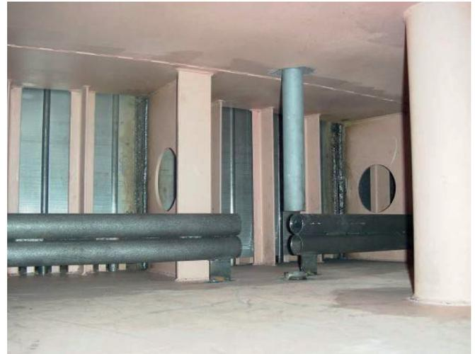
Figure 2: Welded laminated iron core of a Siemens Ring-Motor; view inside the housing
