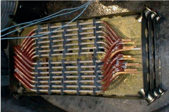
Figure 4: Coils for a GMD during fabrication in the VPI-tank
