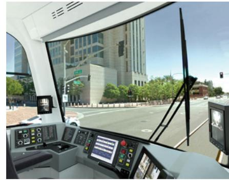
Each streetcar is electrically powered from an overhead catenary system (OCS) and for Orange County operates at speeds up to 44 mph, carrying close to 220 passengers in each vehicle. These streetcars remove automobiles off the road, in turn helping cities decrease their CO2 emissions.
