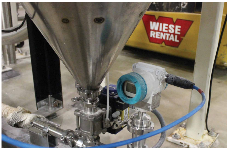
SITRANS P pressure transmitter monitoring the pressure in an eductor.
