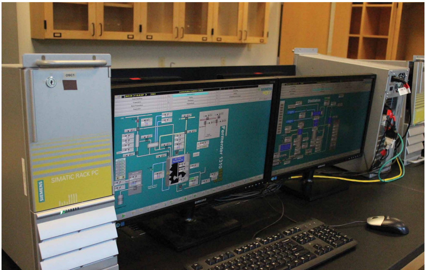
NCERC trains students and new hires using the SIMIT Simulation Platform, which creates a virtual model of a plant’s original PCS 7 control screens.
