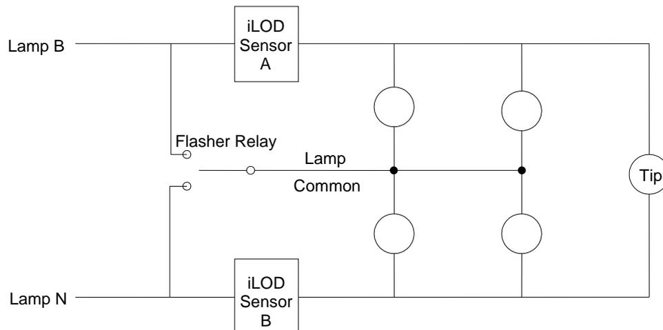
**Figure 9: Correct iLOD Placement in Flasher-Relay Based Crossing Lamp Circuit**
