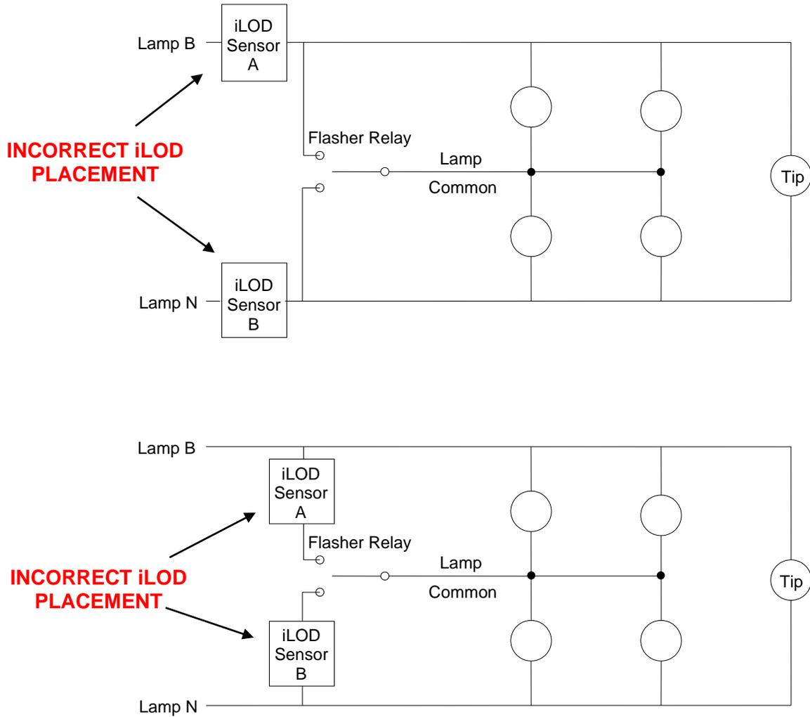
**Figure 10: Incorrect iLOD Placement in Flasher-Relay Based Crossing Lamp Circuit**
