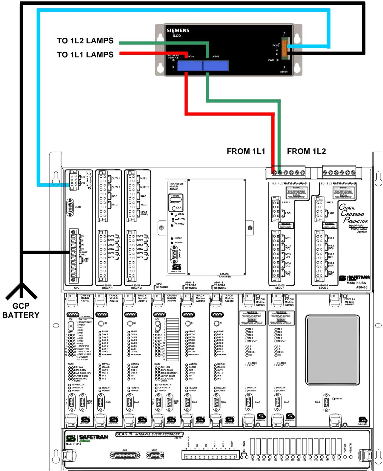
Figure 5: Typical iLOD and SEAR Iii Interconnections
