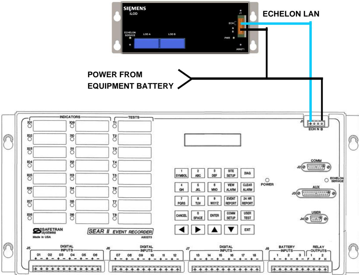
Figure 4: Typical iLOD and SEAR II Interconnections
