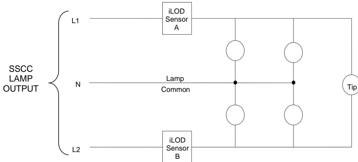
**Figure 11: Correct iLOD Sensor Placement in SSCC Driven Lamp Circuit**
