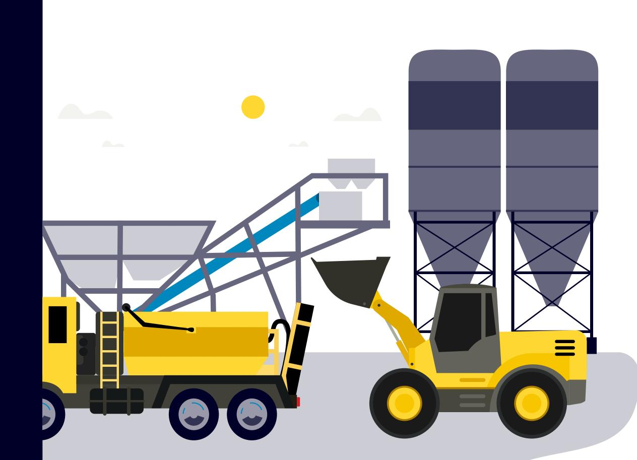
Offsite, a **mobile mixing plant** is producing the raw materials required for construction. The wheel loader shovels the concrete components into a **volumetric lorry** for transit mixing. The lorry makes its way to the construction site with concrete ready for use upon its arrival.
