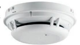
Each detector has two thermal and two optical sensors. This redundancy protects against false alarms caused by deceptive phenomena such as steam, dust, or gas. These detectors are unique in that they offer a No False Alarm Guarantee and also comply with NFPA 76 (Telecommunication Standard) and are classified as a Very Early Warning Fire Detector (VEWFD).
