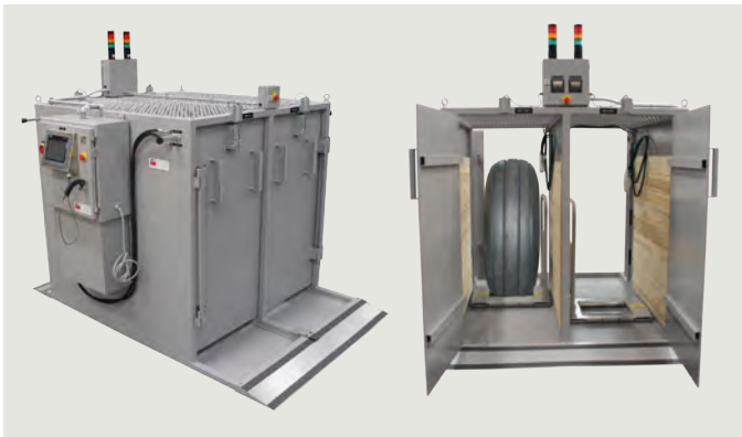
Left, the Bauer 5012 Automatic Tire Inflator fully assembled, with the HMI and barcode scanner visible. Doors are interlocked for safety and process notification. Right, the doors are specially designed to open into the box, to provide protection in the event of a tire failure. Wood absorbs energy in case of a tire failure.
