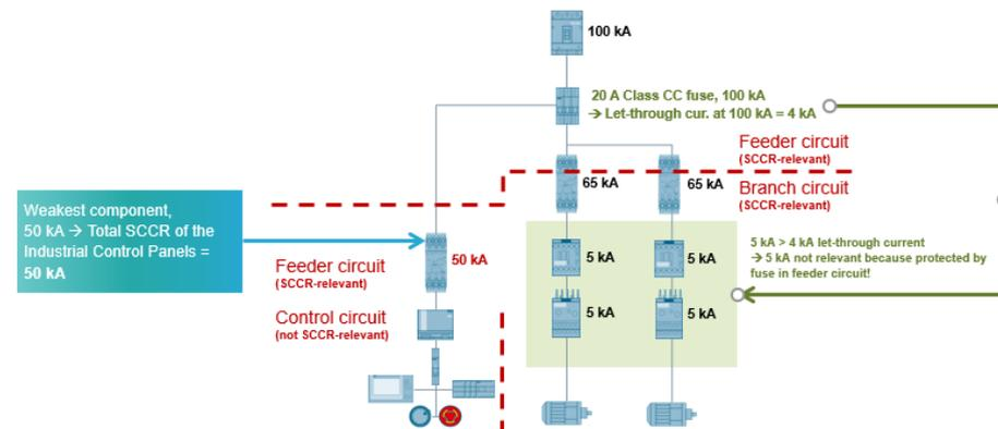
Example 2: SCCR of the industrial control panel **with** current-limiting component in the feeder circuit
