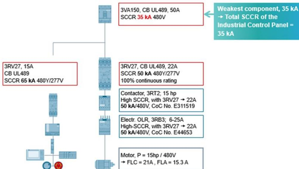
Example of overall SCCR for an industrial control panel
