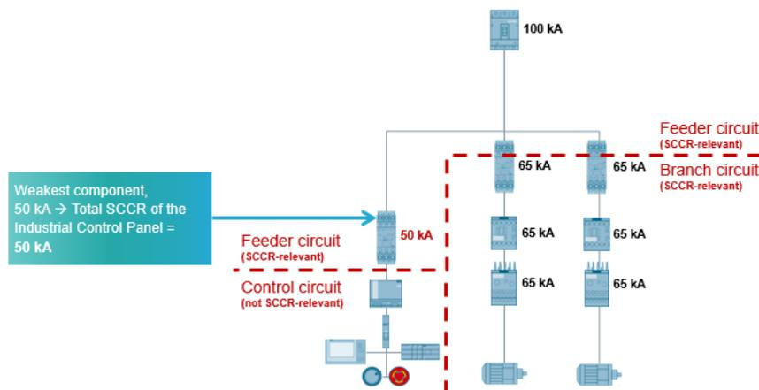
Example 1: SCCR of the industrial control panel **without** current-limiting component in the feeder circuit
