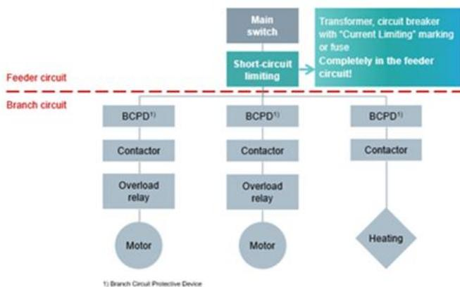
Figure "Short-circuit current-limiting components in the feeder circuit"
