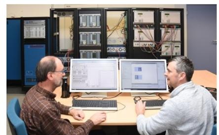
Figure 1: Technical equipment of the simulator (from left to right): RTDS, amplifiers, signal distributor, protection devices
