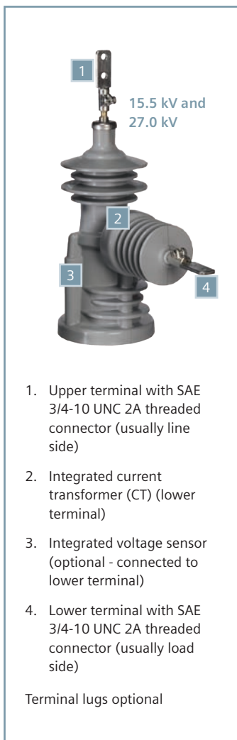
Figure 5: Pole with integrated vacuum interrupter
