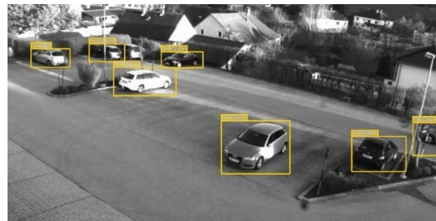
Parking space occupancy monitoring
