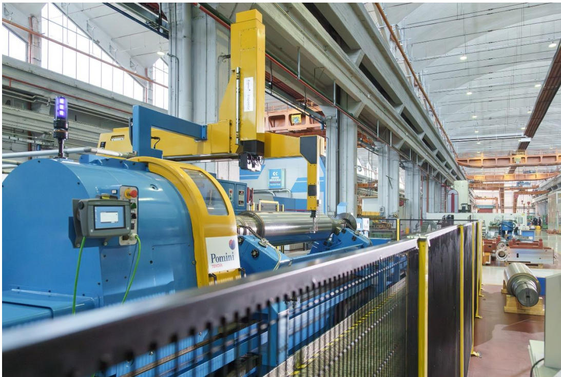
Roll grinder from Pomini Tenova equipped with state-of-the-art CNC and automation technology from Siemens based on Sinumerik One
