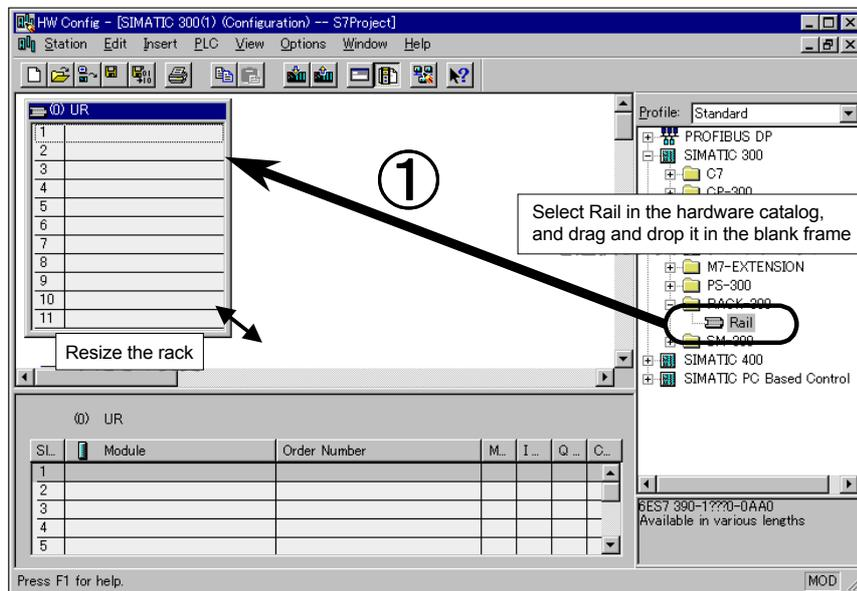
1. Expand the SIMATIC300 category in the hardware catalog to display the S7-300 product groups. Then expand the rack-300 product group to display a rail. Select the rail, and drag and drop it in the blank frame on the left, or simply double-click on the rail. The S7-300 rack will be displayed.
