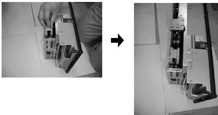
Ensure that the connectors are firmly inserted with their latches fully closed.
