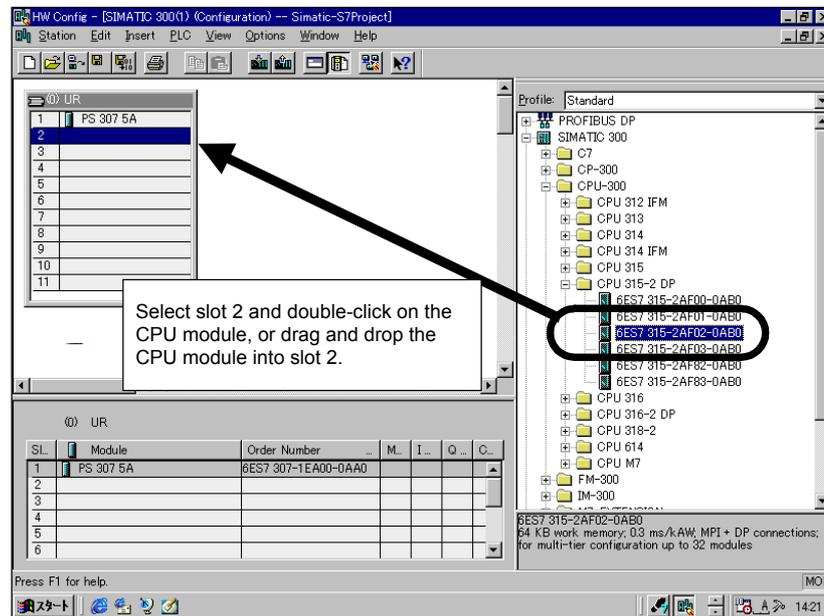
With the S7-300, the CPU module must be inserted in slot 2 of the CPU rack.
