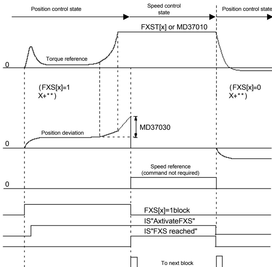
Fig. 14.6 Schema of Fixed Stop function
