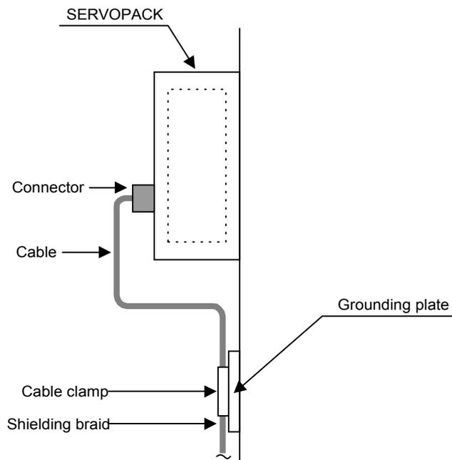
Fig. 2.3 Grounding plate position
