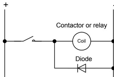
Note: A diode must be installed as close to a coil as possible.
