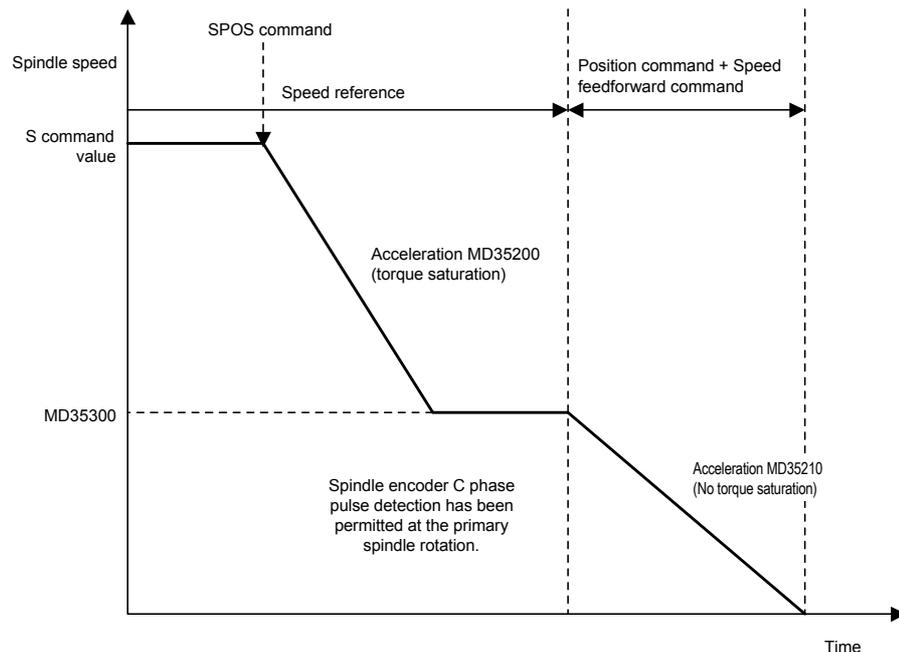
Fig. 14.7 Spindle orientation speed
