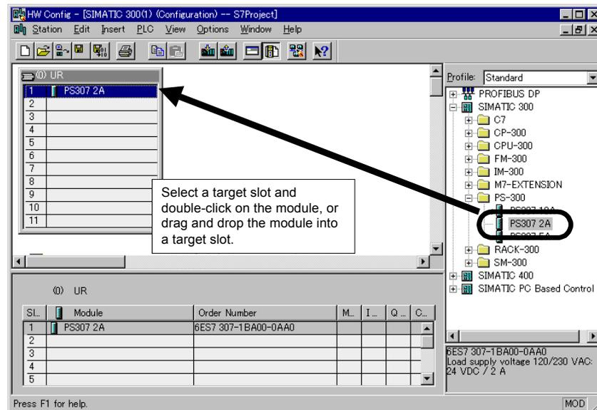
When adding the power supply module, CPU module, or I/O module to the rack, you can use one of the two methods: slot specification and drag-and-drop.
