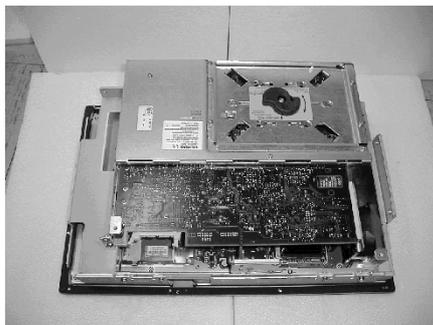
7. Unscrew one M3 screw from the slot cover, and then remove the slot cover.
