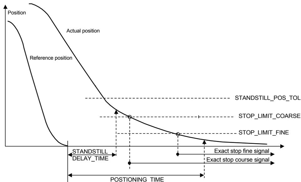
Fig. 14.3 Positioning timing
