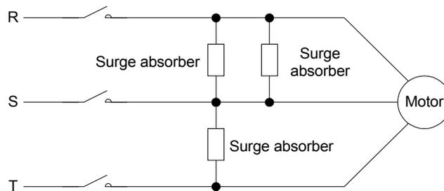
Note: A surge absorber must be installed as close to a motor as possible.
