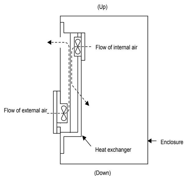
Fig. 2.1 Example installation of a heat exchanger
