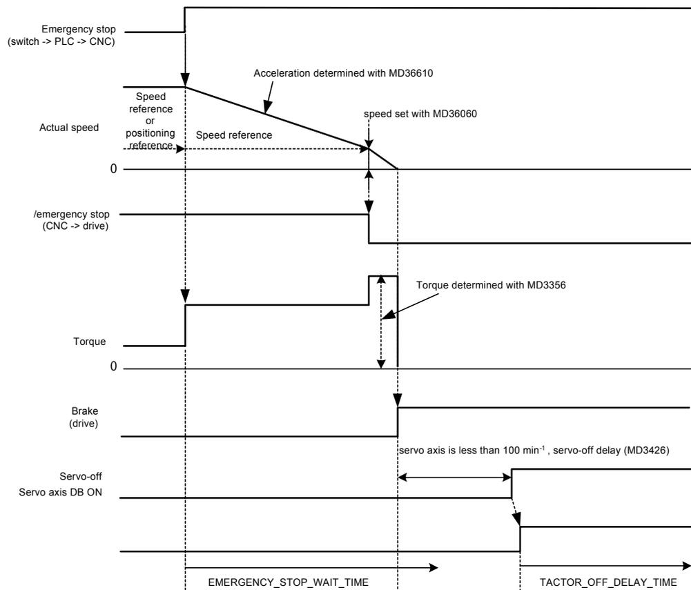
Fig. 14.4 Emergency stop processing
