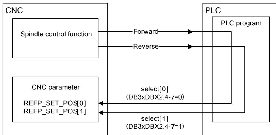
Fig. 14.8 Spindle orientation C phase range compensation
