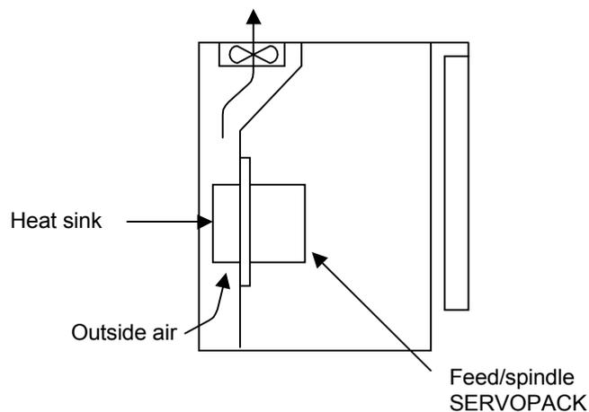
Fig. 2.5 Heat sink as exposed to the outside
