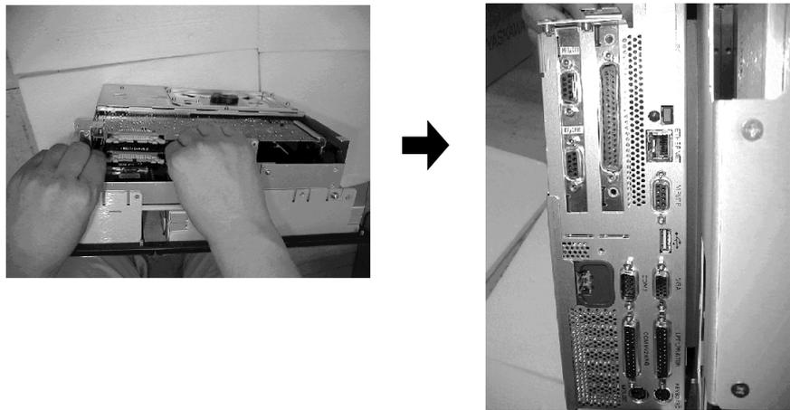
10. Connect the MCI Extension Board connector to the corresponding connector on the board above it using the supplied cable.
