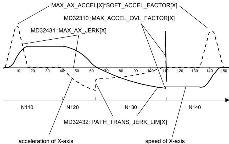
Fig. 14.2 Function of machine data related to acc./dec.
