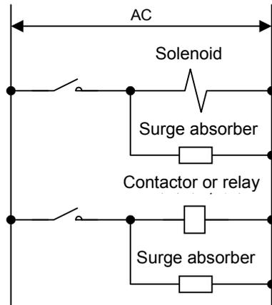
Note: A surge absorber must be installed as close to a coil as possible.
