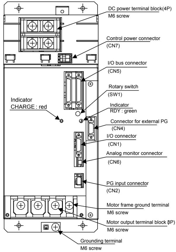
■ 1-axis servo unit (SGDK-50AEA (5 kW))
