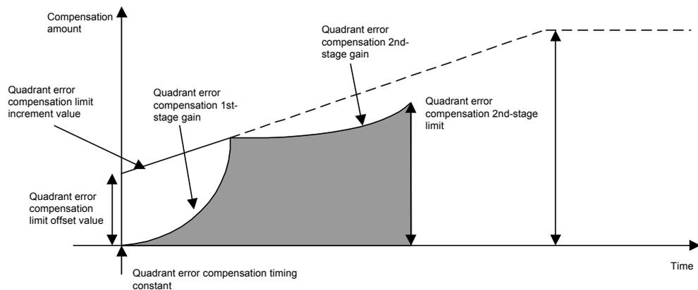
Fig. 14.1 Functional quadrant error compensation waveform
