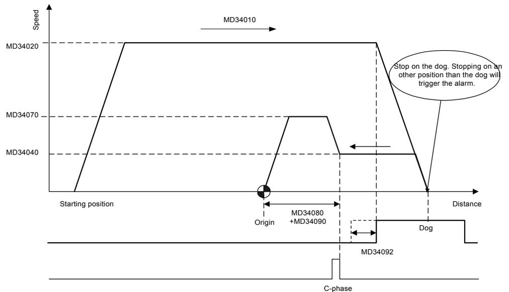
Fig. 14.5 Schema of return to reference point action
