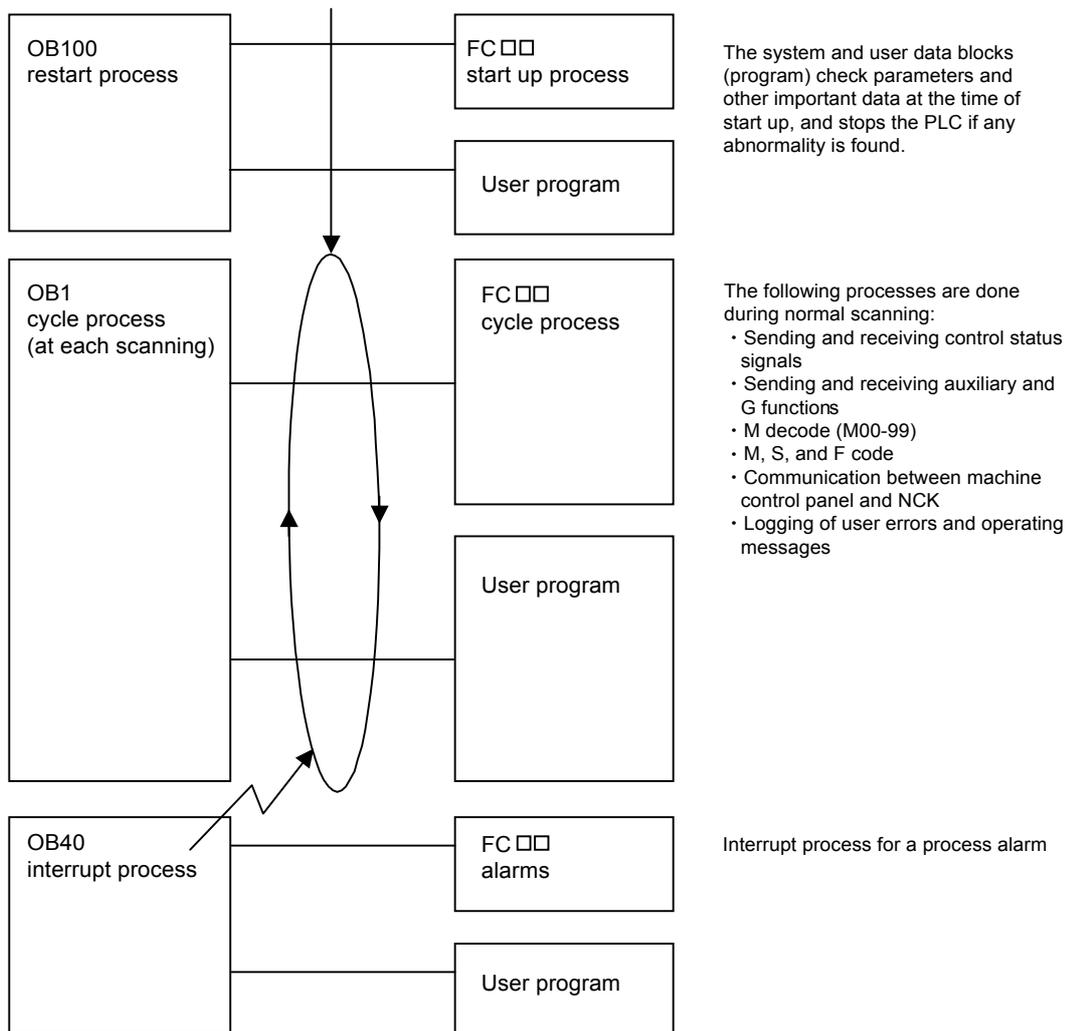
The illustration above shows only basic the parts of a program. An actual program may be more complicated including some other interrupt processes. For details on OB, FC and FB, see the System Software for S7-300/S7-400 (System and Standard Functions).
