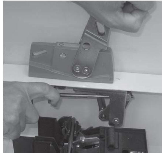
Figure 9 Defeating Cover Catch Interlock
