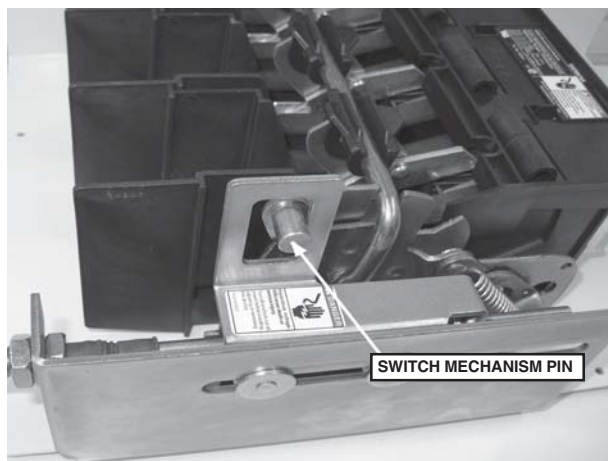
Figure 8 Installation of Switch Mechanism Pin Into Slide Plate Operator Slot
