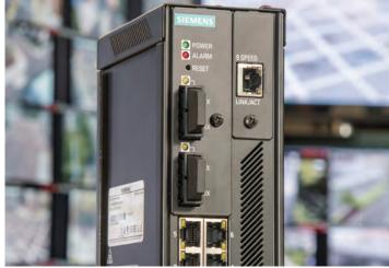
Stamford's resulting ITS network relies on two RUGGEDCOM RX5000 multi-service platforms with high port density at each hub to provide redundant support to RS900 managed Ethernet switches for traffic signal monitoring and control and to support RSG2200s, 9-port managed gigabit Ethernet switches that handle each intersection's video feeds.
