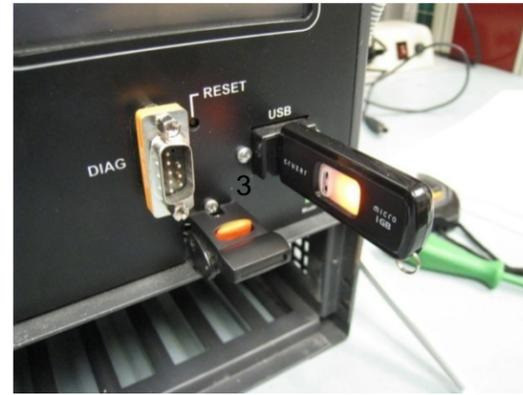
3. Within a few seconds after inserting the USB Drive the USB Wizard main menu will appear on the display (figure #1). Press the **Reset Button** (figure #2) located to the left of the USB port on the Display II Module front panel.
