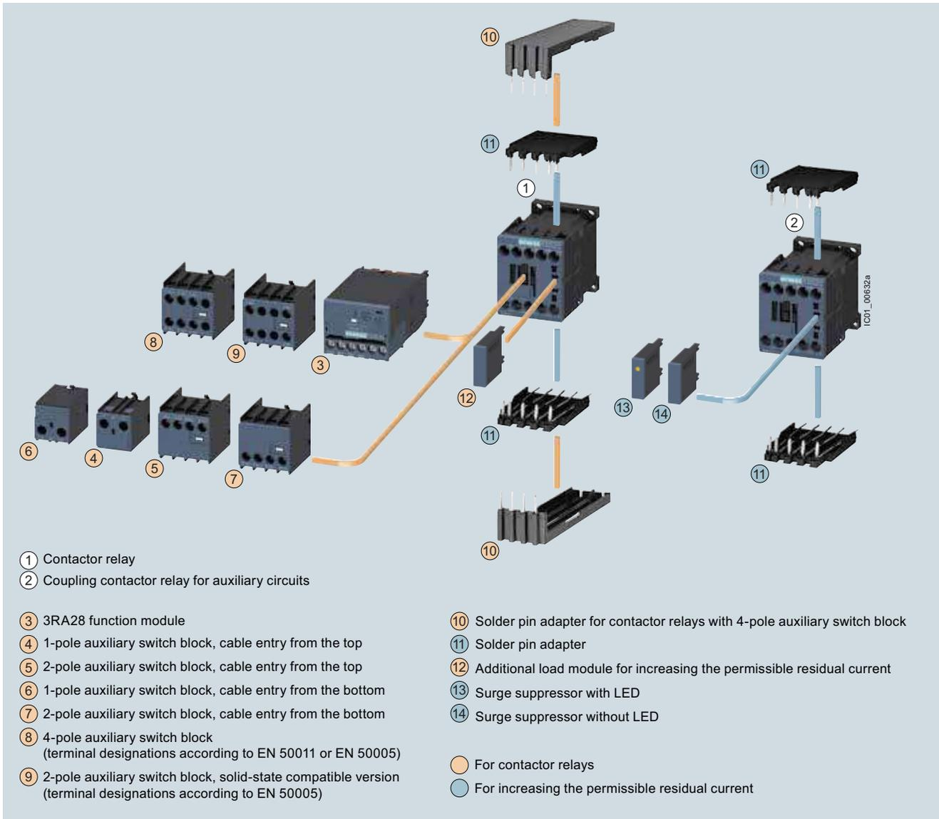
3RT2 contactors and coupling relays – Size S00 with mountable accessories
