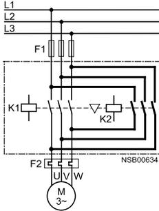
The 3RA2913-2AA. (S00) and 3RA2913-2AA (S0) installation kit contains wiring connectors for connecting the main conducting paths, the mechanical interlock and two connecting clips for the contactors.
