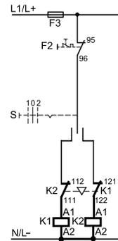
The 3RA19 24-2B mechanical interlock contains one NC contact for the NC contact interlock for each contactor
