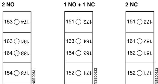
**3RH19 21- . KA.. second laterally mountable auxiliary switch blocks (right)**
