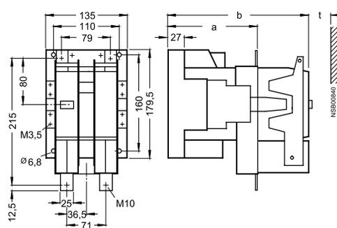
t = minimum clearance from insulated components: 20 mm (600 V and 750 V)
