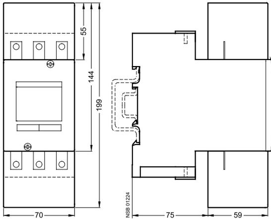
Auxiliary conductor terminal, 3-pole
