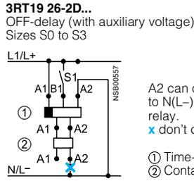
A2 can only be connected to N(L-) via the time-delay relay.
