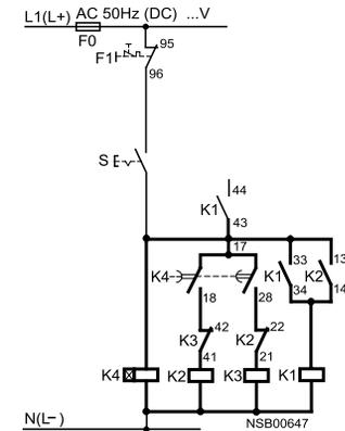
Contact element 17/18 is only closed on the star step; the contact element is open on the delta step and when de-energized.
