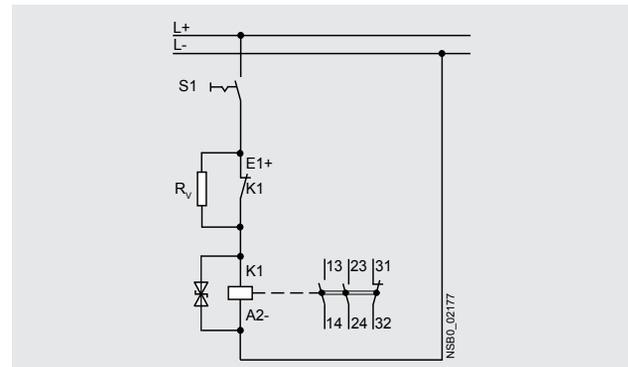
A 4-pole auxiliary switch block (according to EN 50005) can be fitted additionally.
