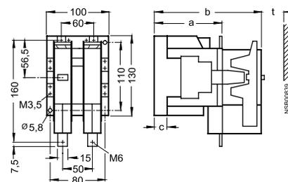
t = minimum clearance from insulated components: 15 mm (600 V), 20 mm (750 V)
