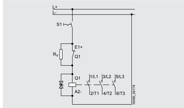
The size S00 contactors are supplied prewired with a plug-on module containing the series resistor. The suppressor diode is integrated. A 4-pole auxiliary switch block (according to EN 50005) can be fitted additionally.
