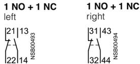
**3RH19 21-...JA11, 3RH19 21-2JE11 second laterally mountable auxiliary switch block (solid-state compatible)**
