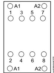
Size S0 with integrated 1NO + 1NC aux (13/14 + 21/22) and only one set of A1+A2 on front
