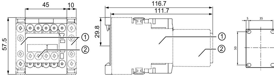
Lateral clearance from earthed parts = 6 mm
