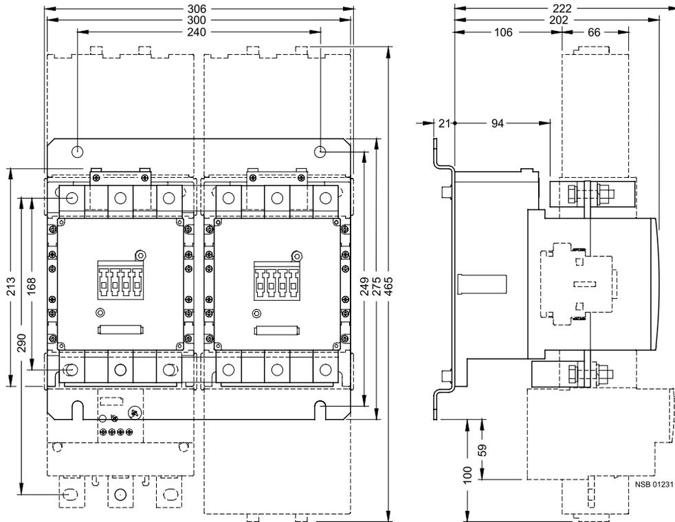
The assemblies shown on this page are for customer assembly with individual components.
