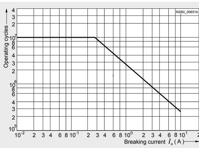
Contact erosion indication with vacuum contactors
