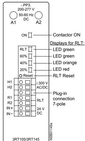
To supply power to the solenoid operating mechanism and the remaining lifetime indication, the control supply voltage  $U_s$  must be run to terminals A1/A2 of the laterally mounted electronics module. The control inputs of the contactor are brought out to a 7-pole plug-in connection; the connector, using screwless spring-force technology, is included in the scope of supply.
