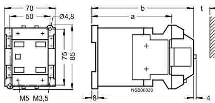
t = minimum clearance from insulated components: 15 mm (600 V and 750 V)
