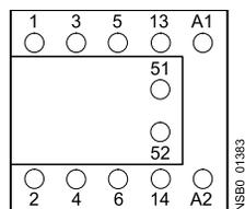
The auxiliary switch block comprises 3 leading contacts (not shown) and one unassigned NO contact.
