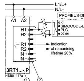
Electronics module of 3RT1 ...-P contactor
