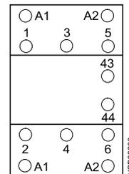
The auxiliary switch block comprises 3 leading contacts (not shown) and one unassigned NO contact.
