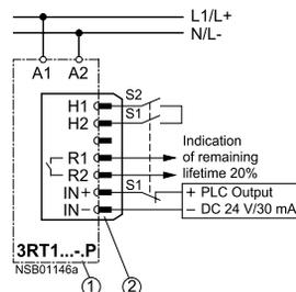
Electronics module of 3RT1 ...-P contactor
