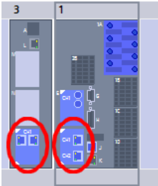
Figure 5-106 Insertion Position for a USART Module
