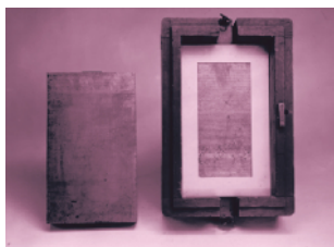
PLATE-TYPE LIGHTNING CONDUCTORS for the Berlin–Frankfurt am Main Telegraph Line, 1849.
