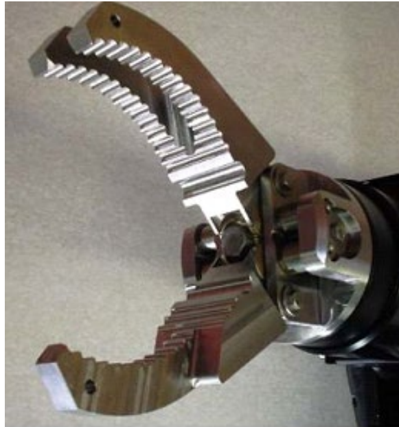
Figure 19 - Recommended ROV Manipulator Jaw for Fishtail Handle
