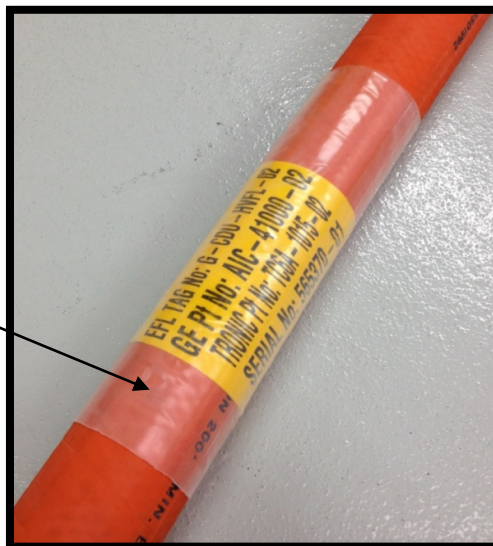
Figure 2 – Marking of Hoses
