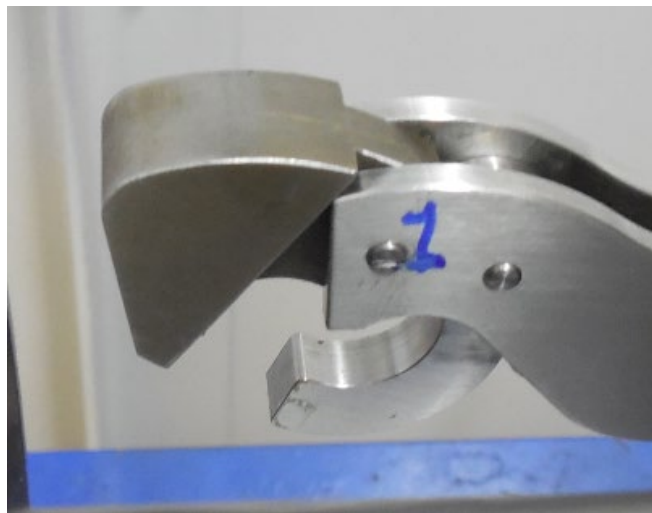
Figure 28 - Lock after Emergency Release
