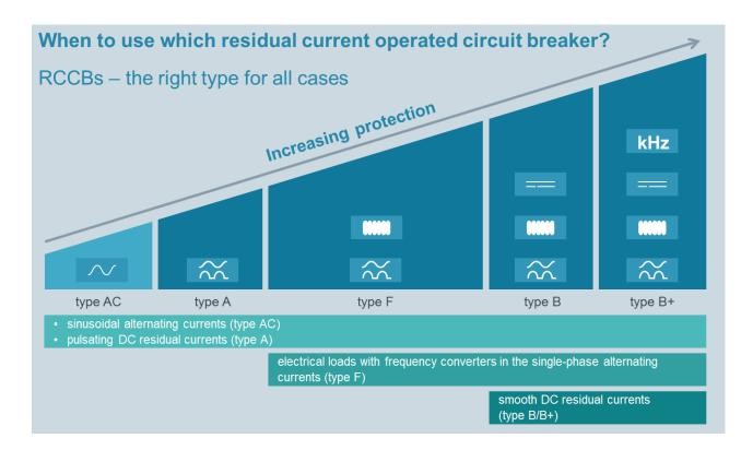
5SV3 RCCBs Type B/B+ are used in devices such as frequency converters, medical devices and UPS systems. Smooth DC residual currents or currents with low residual ripple may occur in the event of a fault on these devices. RCCBs type A are unable to detect these smooth DC residual currents.
