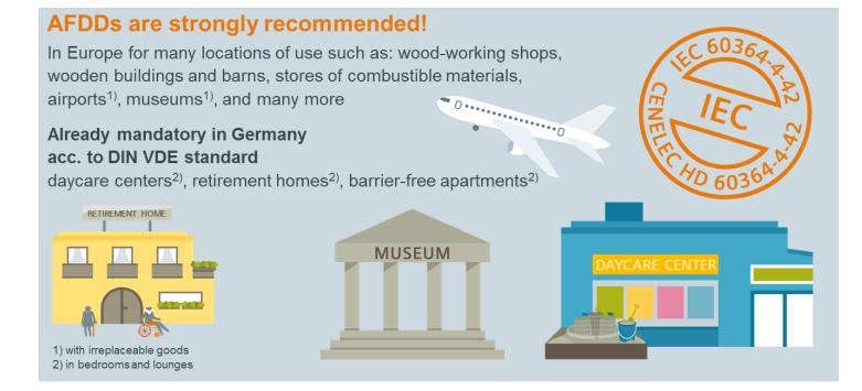
Specifically: In all electrical installations planned after publishing the current version of DIN VDE 0100-420 in February 2016, the installation of arc-fault protection devices is mandatory in the defined areas of application.
