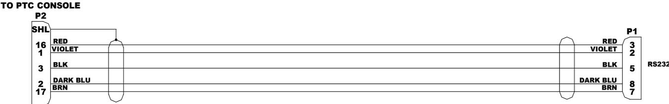
Figure 1-6 A26775-0X MultiPort Cable Wiring Diagram
