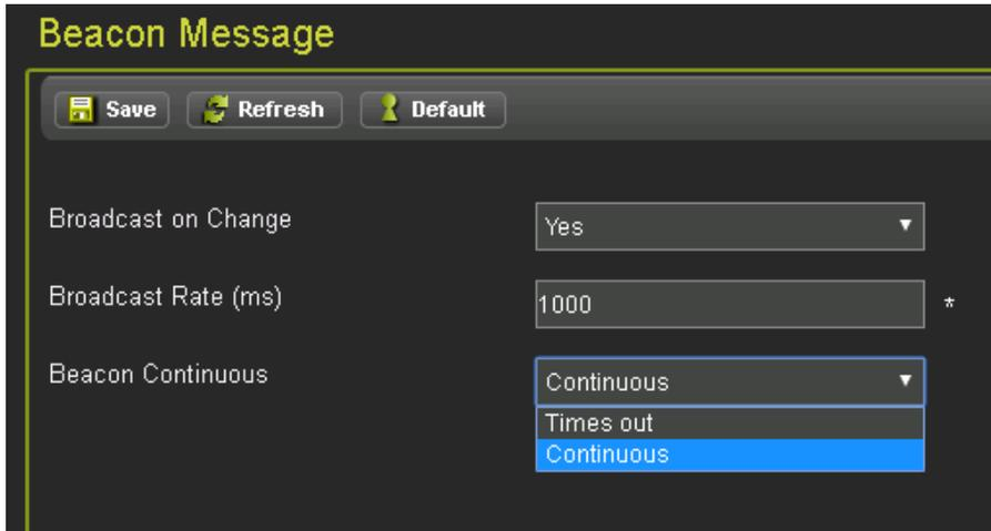
**Figure 4-13 PTC - Beacon Message Configuration - Beacon Continuous**
