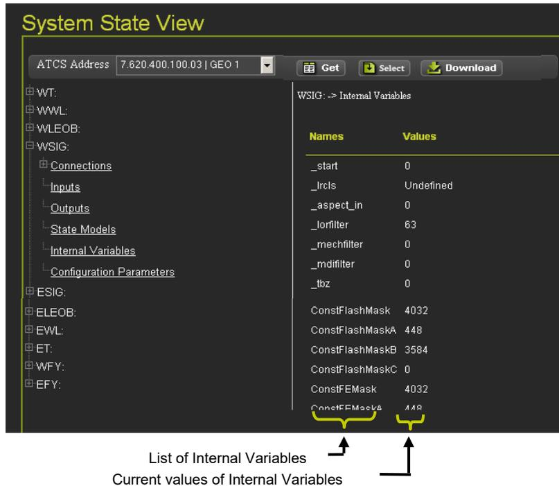
**Figure 4-81 System State Views - Internal Variables**
