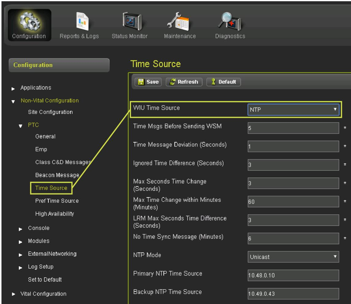
**Figure 4-16 PTC - Time Source Configuration - NTP Option Parameters**
