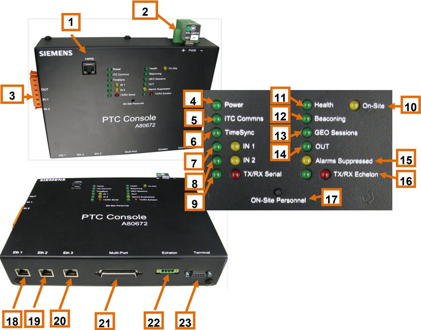
Figure 1-2 PTC Console Indicator and Controls Locations
