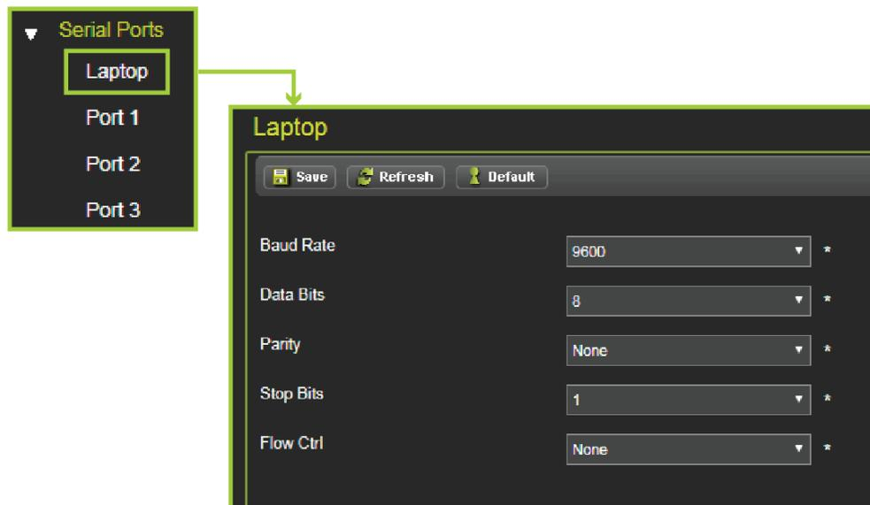
**Figure 4-23 Configuration Serial Ports**
