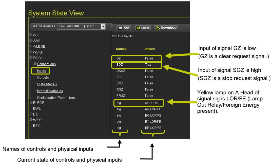
**Figure 4-78 System State View - GEO Inputs**
