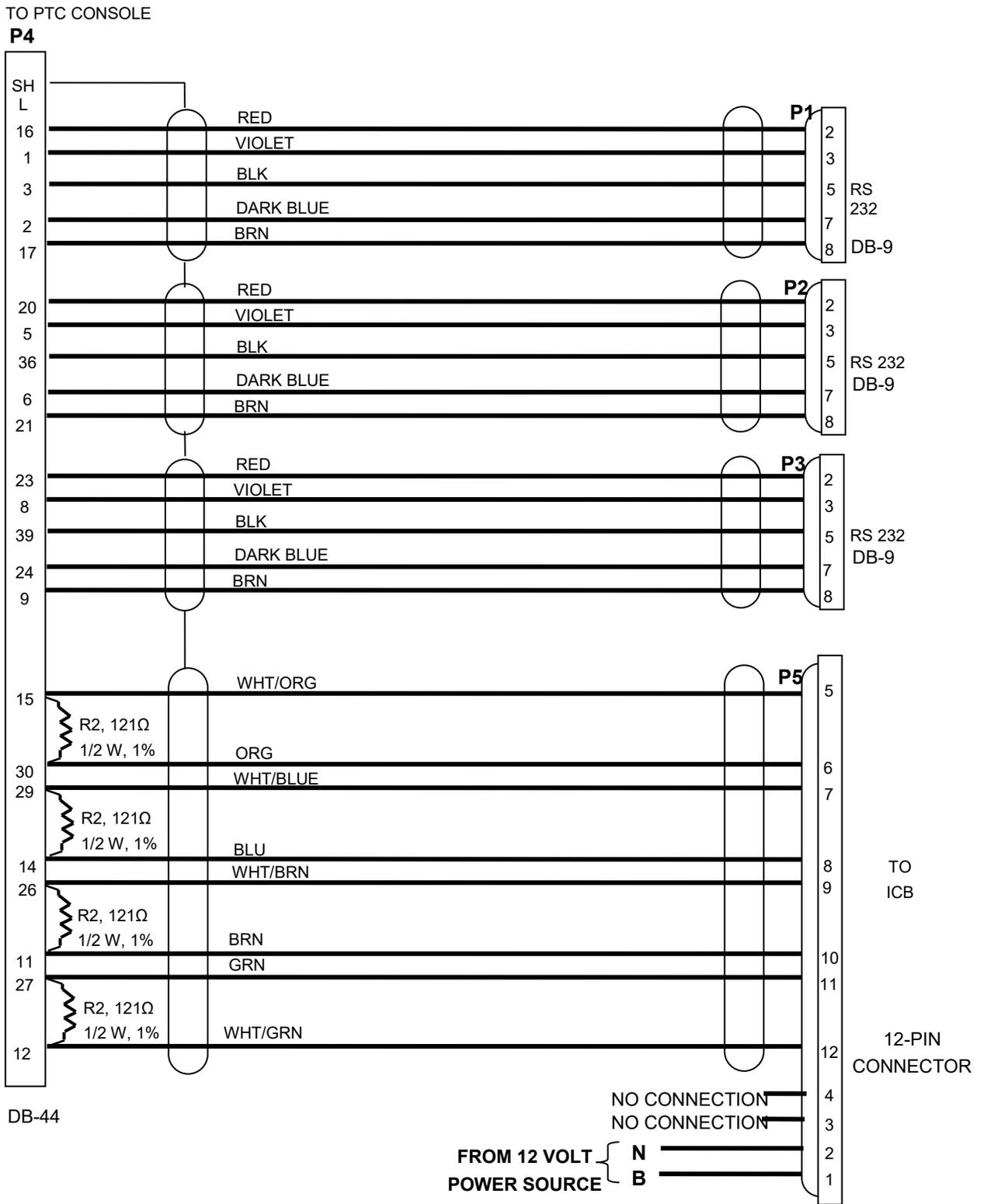
Figure 1-4 A26702-0X MultiPort Cable Wiring Diagram
