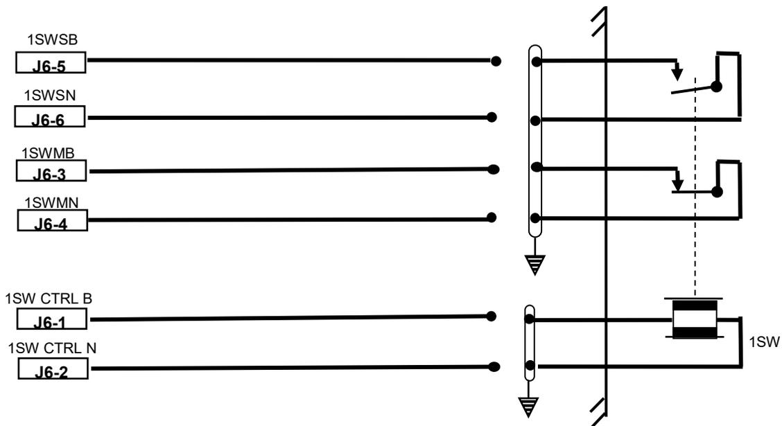
Figure 3-5 Example Dark Territory Switch Monitor Wiring Diagram
