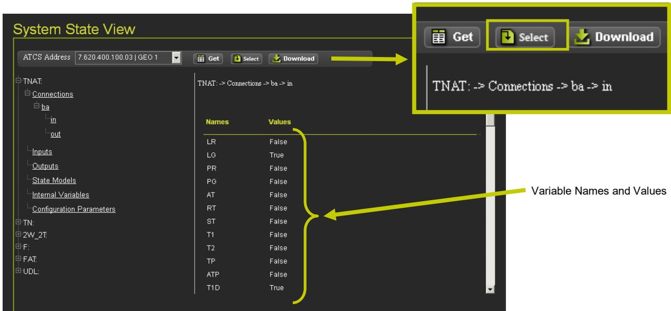
**Figure 4-75 System State View - View Object Values**
