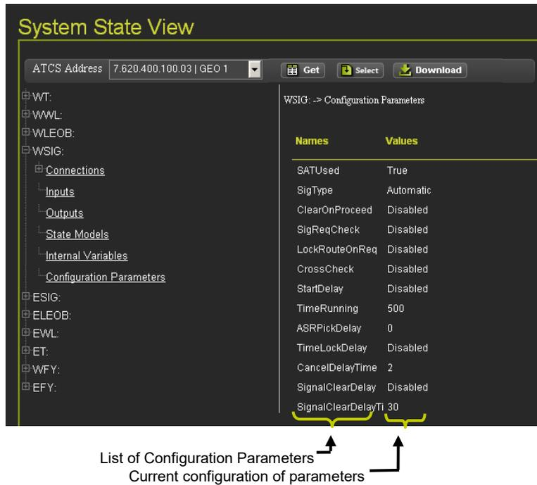
**Figure 4-82 System State Views - Configuration Parameters**
