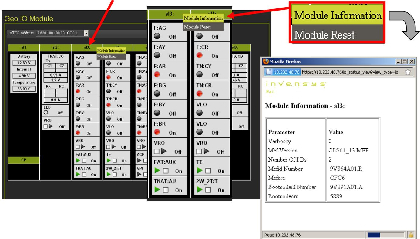
Figure 4-93 GEO I/O - GEO Module Information
