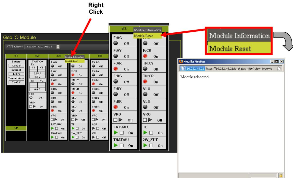
**Figure 4-94 GEO I/O - GEO Module Reset**
