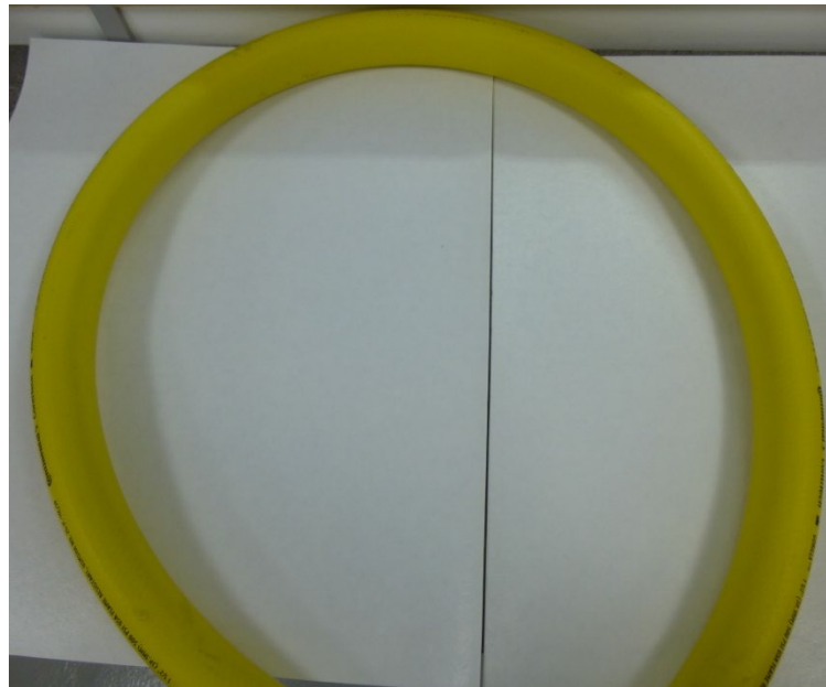
Figure 13- MBR being maintained (Gorilla 1.5" Hose)
