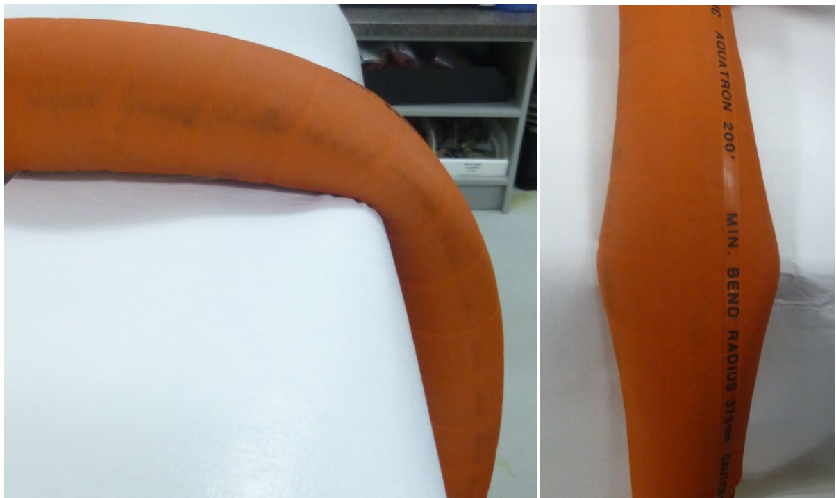
Figure 14-Incorrect routing (hose deformed over "sharp" edge- AquaTRON 200 Hose)
