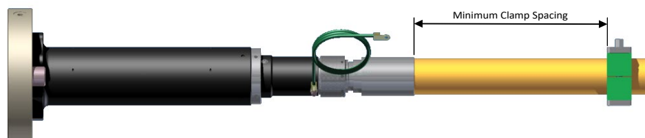
Figure 22 - Minimum clamp spacing from connector
