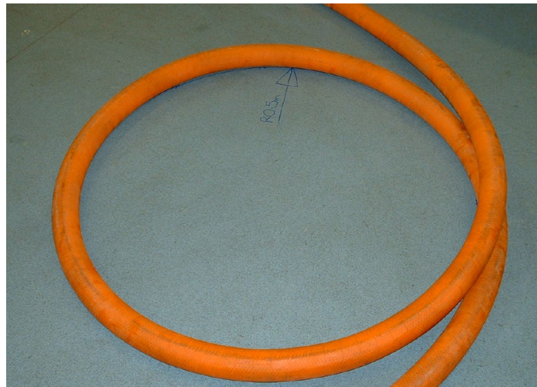
Figure 12-MBR being maintained (AquaTRON 200 Hose)
