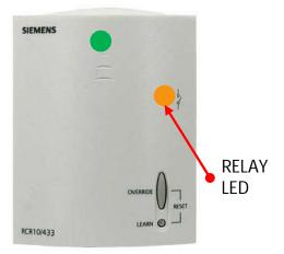
The thermostat and receiver are now paired. To test the signal press the TEST button on the back of the room thermostat for 1 second and release. The Relay LED Will flash <a href="MBER">AMBER</a> and stay on. To deactivate press the TEST button again, the relay LED will flash <a href="AMBER">AMBER</a> and go blank.
