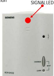
Next put the RCR10/433 in learning mode. Press the LEARN button for 1 second and release. The signal LED will flash AIMBER to confirm learn mode is active and go blank.
