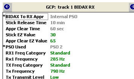
Figure 56: GCP: track “n” BIDAX RX/TX
