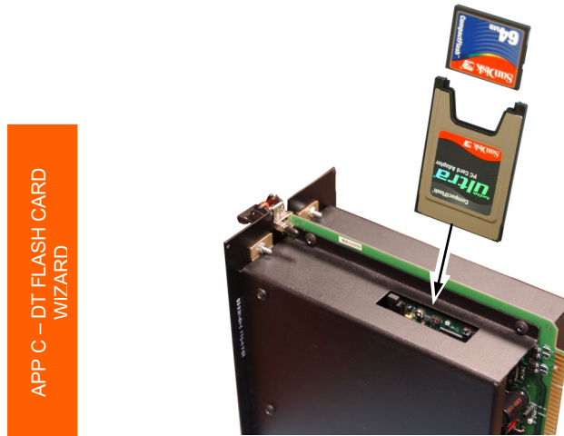
Figure 200: Display Module with CompactFlash® Card
