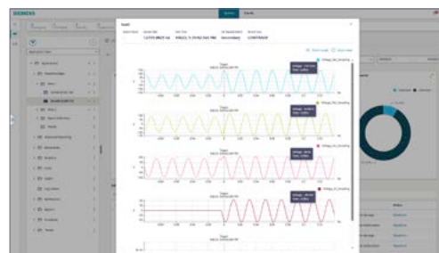
Voltage events: detailed waveform for in-depth evaluation
