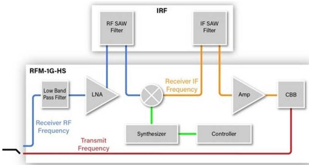
Figure 2-4 RF and IF SAW Filters
