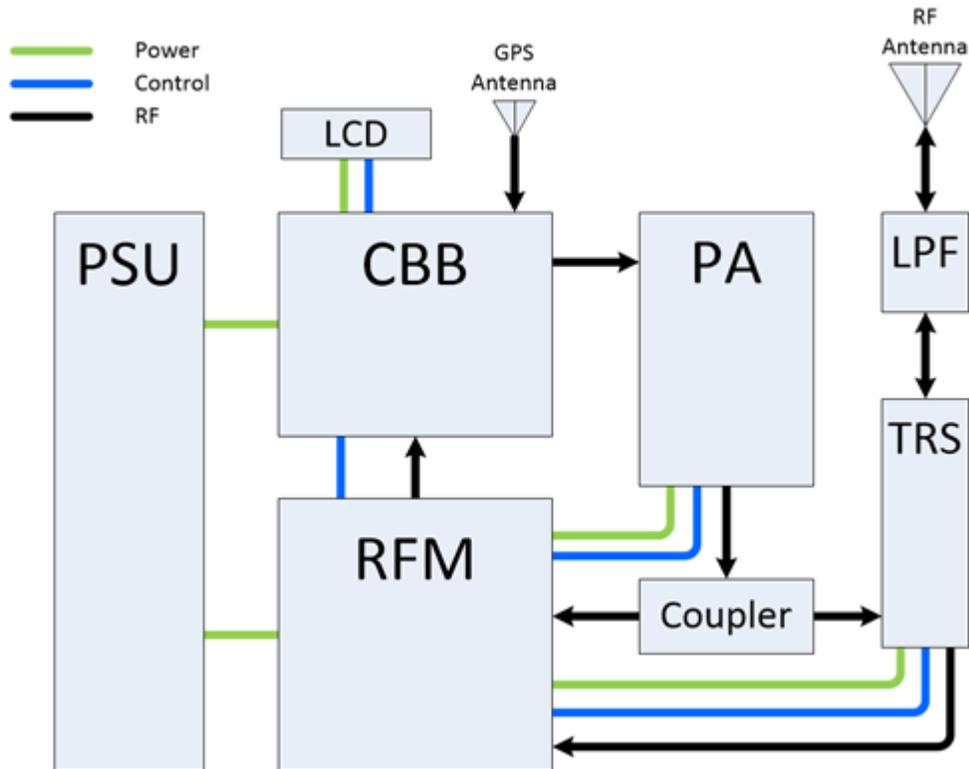
Figure 2-3 Airlink Mars Radio Block Diagram
