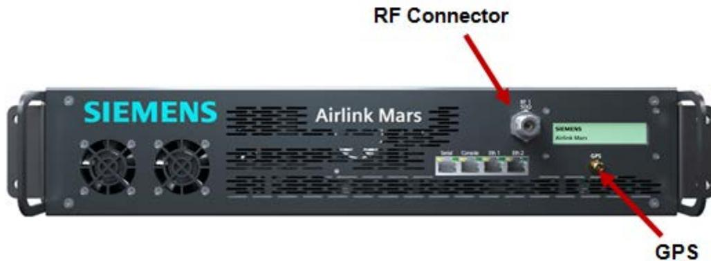
Figure 3-5 Antenna Connections
