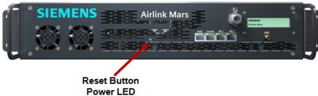
**Figure 3-4 Power LED and Reset Button**
