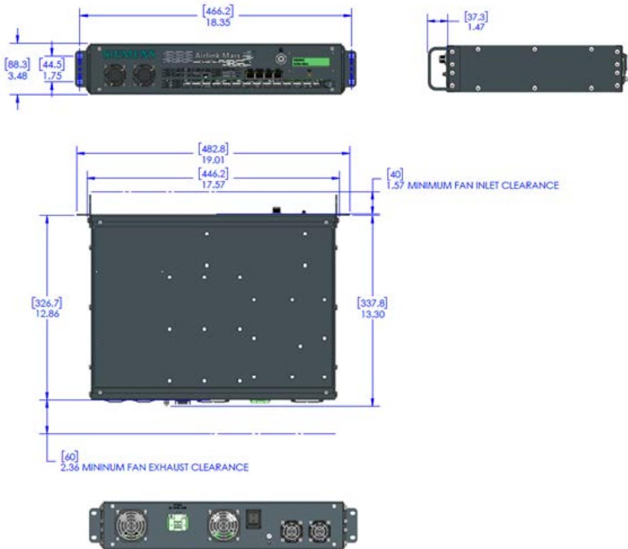
Figure 2-2 Airlink Mars Radio Dimensions
