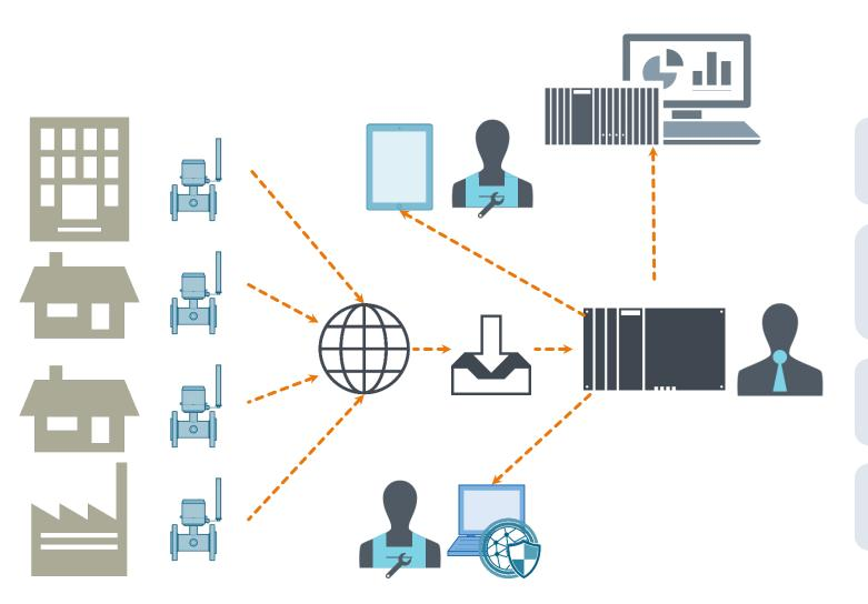
The measurement data can be accessed over the Internet with a web browser on PC or smart device.
