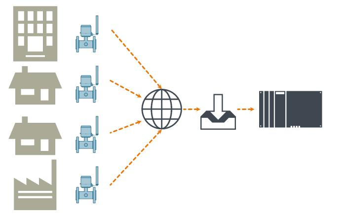
Through the Wireless Module, the measurement data in MAG8000 are accessible remotely via cellular network.
