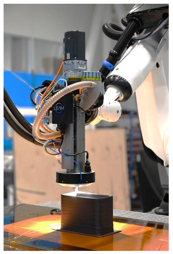
LEAM Technologies is revolutionizing large format additive manufacturing (LFAM) with light-based welding technology.
