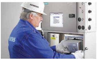
An entirely new Maxum oven option is available where all the components of the measurement including the valves, columns and detectors are mounted on a single, removable module enabling the repair of the entire analytics back in the convenience of the user's maintenance shop.
