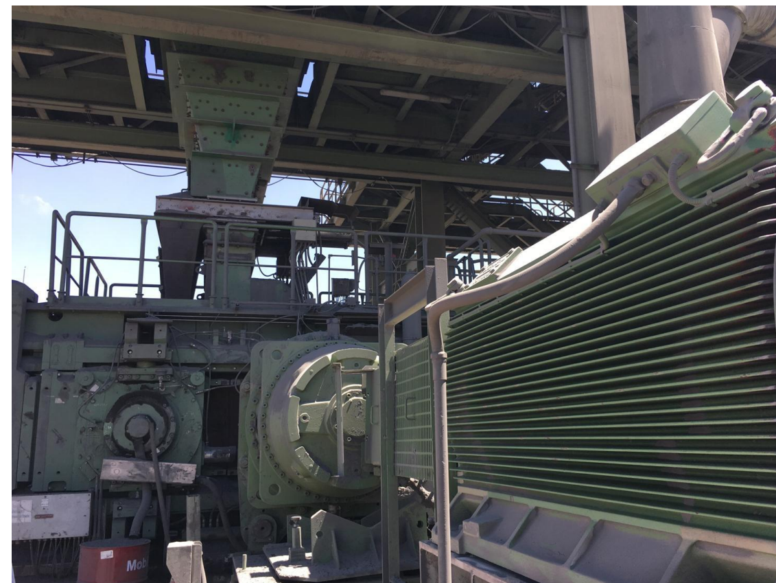
H-Compact Motor 1870 kW 4.0 kV High pressure grinding rolls application
