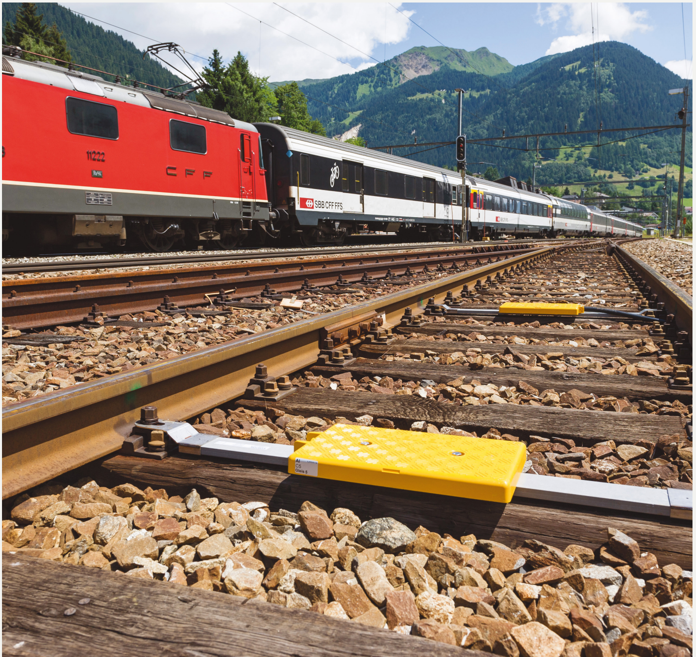
Balises installed in the track bed communicate with the on-board computer via the air interface and with the trackside MiniLEU by cable.
