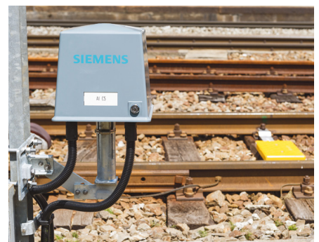
Smart combination for the ETCS safety standard: Trainguard MiniLEU S11 and Trainguard Eurobalise S11
