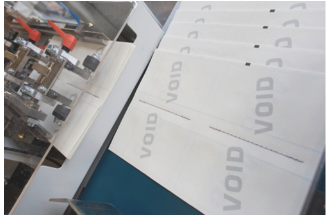
The process results in booklets, sewn in two-up production, and checked for the correct collation of the individual sheets, ready for further processing.
