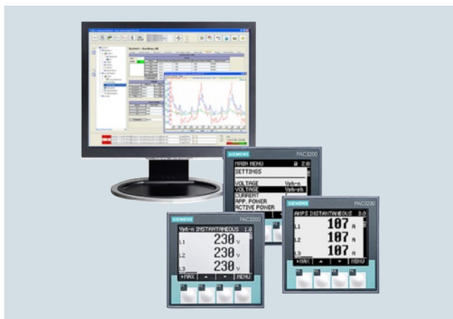
Components of the PC-based power monitoring system
