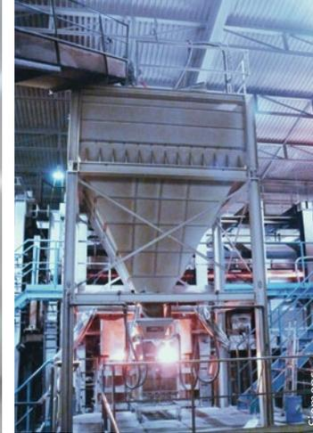
The LR560 radar level measuring device is installed in the day silo, which ensures a continuous supply of batch material for the melting furnace.
