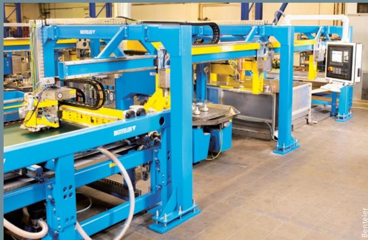
drill automotive glass. The lines have a modular design and can therefore be extended easily by one or more sections. The company's lines are now equipped with the premium CNC controllers Sinumerik 840D sl and the latest drive technology from Siemens.
