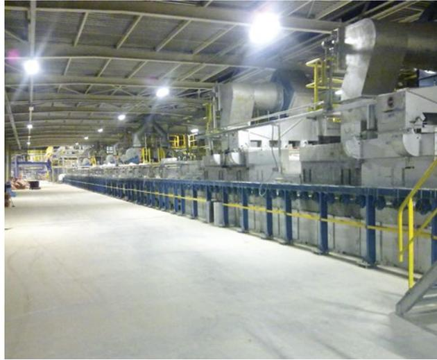
A glimpse into the plant (from left to right): float glass furnace, tin bath and annealing lehr at CFG in Dagestan, installed by Horn Glass, which took on all production line technology as general contractor.
