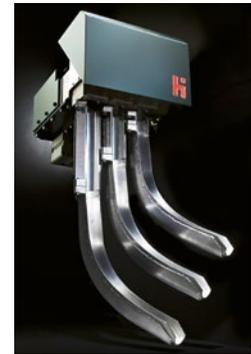
Whether operating the plunger, dual motor shears or gob distributor (from top to bottom): the Simotion Servodrive can control the various hot end components with precision.
