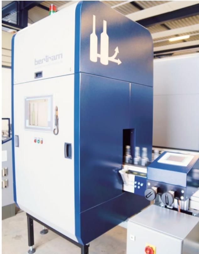
The Separator divides different types of bottles and glass containers into as many as four streams, all while maintaining consistent production speed.
