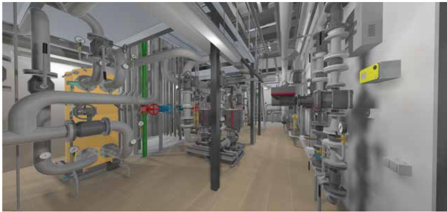
Ecodomus supports multiple rendering quality options, merging of 3D parametric models (produced from BIM) with point clouds and CityGML files within the same scene.
