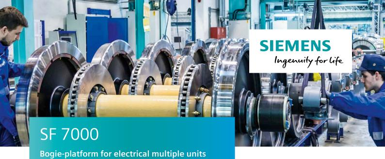
The bogie SF 7000 was developed especially for the UK market to equip regional trainsets for speeds of up to 160 km/h.
