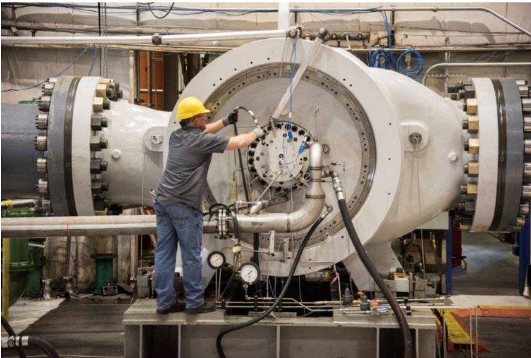
RFBB36 pipeline compressor.
