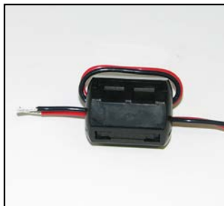
Figure 2-7 EMI Filter Installed
