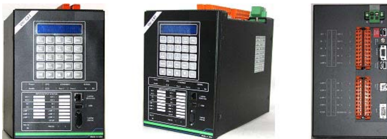
Figure 1-1 Vital Interface Unit – Coded Audio Track (VIU/CAT) Front, Oblique, Top Views
