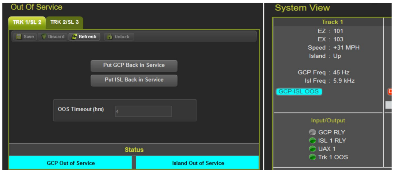
Figure 4-6 Island Out of Service Indications on WebUI
