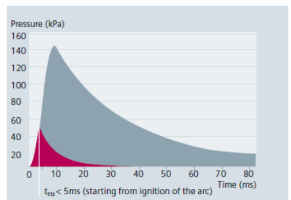
Figure 3 Sample pressure curve in a compartment for an internal arc fault current of 80 kA (peak) / 31.5 kA (rms)
