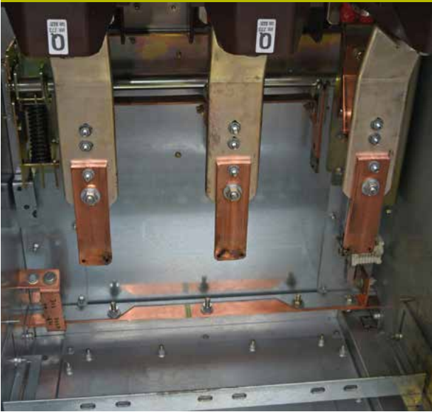
Fig. 4 Condition of a 12 kV NXAIR cable compartment after an internal arcing test with a fault current of 80 kA (peak) / 31.5 kA (r.m.s.), with arc ignition inside the cable compartment
