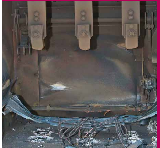
Fig. 4 Condition of a 12 kV NXAIR cable compartment after an internal arcing test with a fault current of 80 kA (peak) / 31.5 kA (r.m.s.), with arc ignition inside the cable compartment
