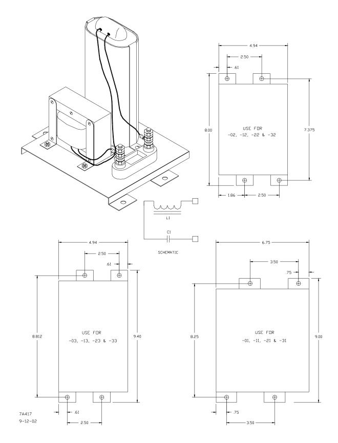
Figure 5-9 PSO Cab Signal Filter, 7A417-X, With Mounting Dimensions
