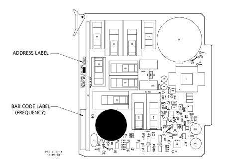
Figure 6-2 Location of Transmitter Module Address and Frequency Labels
