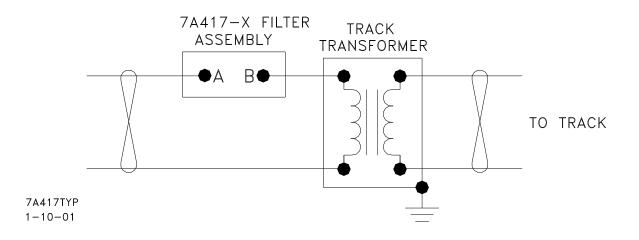
The 7A417-X filter assembly can be configured according to signal frequency and relay mounting base type as indicated in the tab chart below. See figure 5-9 for mounting dimensions.
