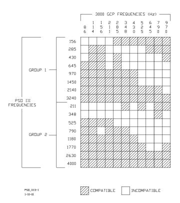
Figure 3-1 PSO III And 3000 MS/GCP Frequency Compatibility
