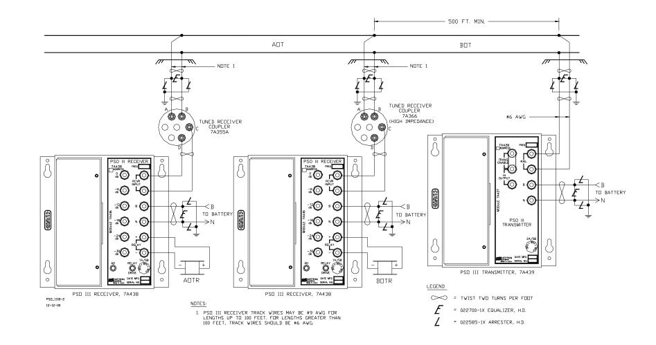
Figure 8-2 PSO III Installation With Tuned Receiver Coupler, 7A366-f
