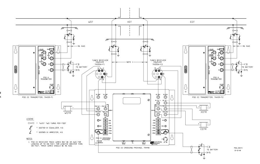
Figure 8-5 Typical Installation of PSO III Crossing Package With Island Circuit
