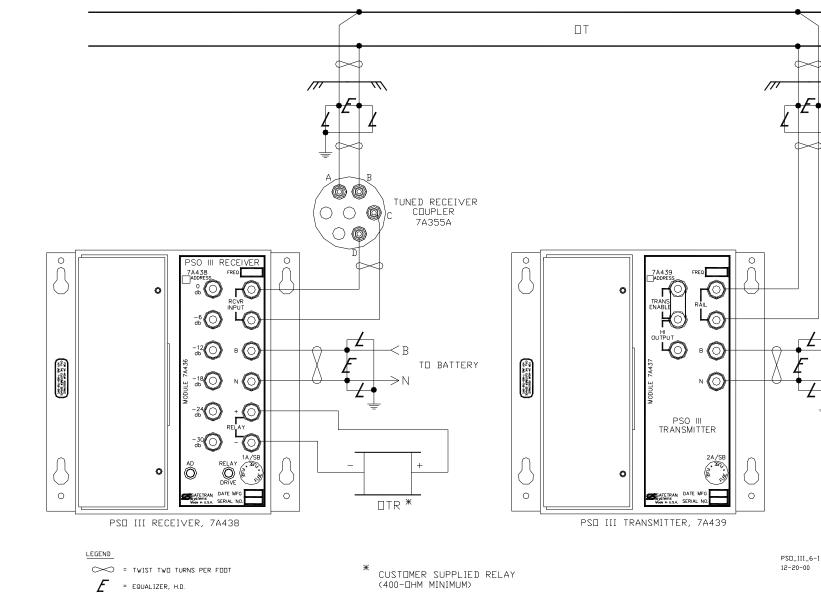
Figure 6-1 Typical PSO III Installation
