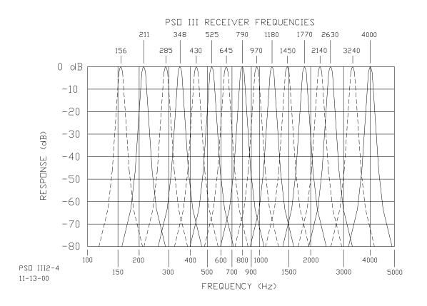
Figure 2-4 Typical Receiver Frequency Response Curves
