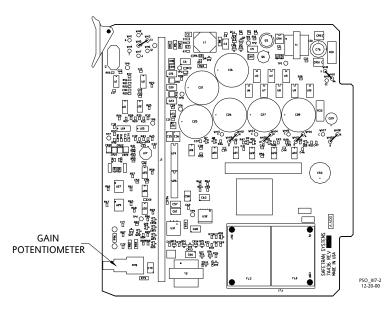
Figure 7-2 Gain Potentiometer Location On 7A436 Receiver Module
