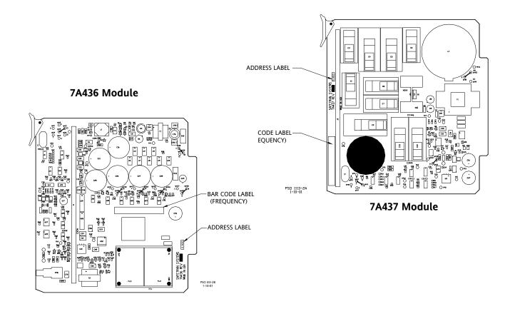
Figure 3-2 Address Code and Bar Code (Frequency) Label Locations, 7A436 And 7A437 Modules
