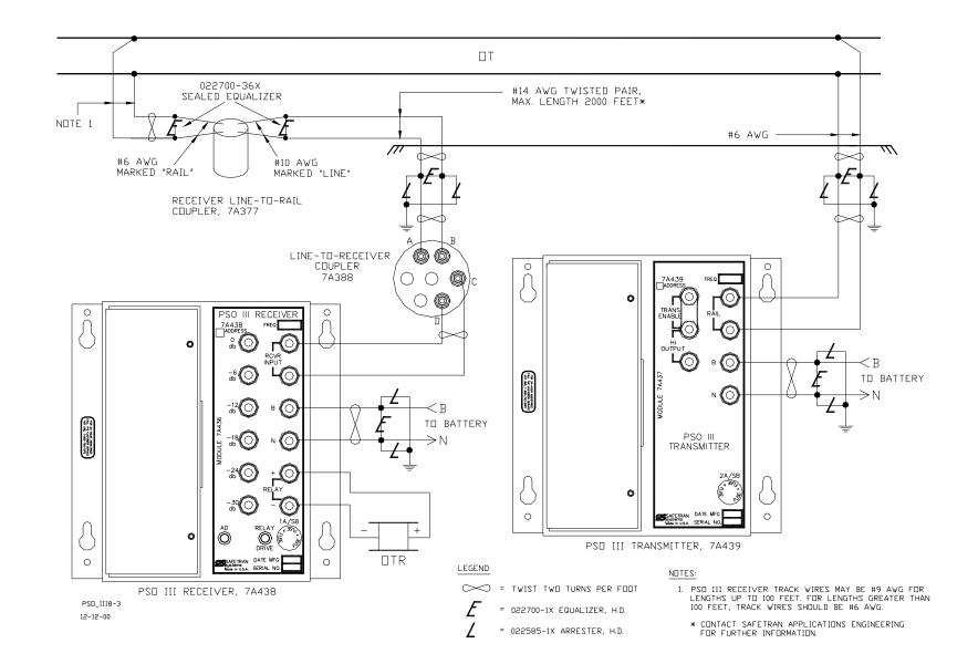
Figure 8-3 PSO III Installation With Receiver Line-To-Rail Coupler, 7A377-1-f, And Line-To-Receiver Coupler, 7A388
