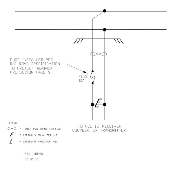
Figure 8-10 Typical Track Wire Surge Protection For Use In Electrified Territory
