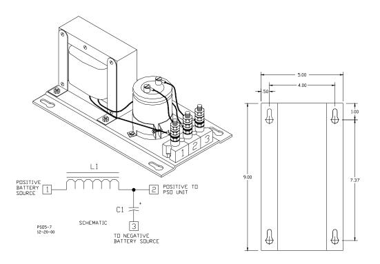
Figure 5-7 Battery Line Filter, 7A418, With Mounting Dimensions
