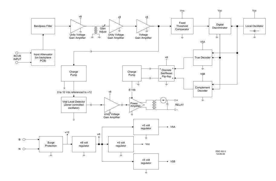
Figure 2-3 Receiver Assembly, 7A438, Block Diagram
