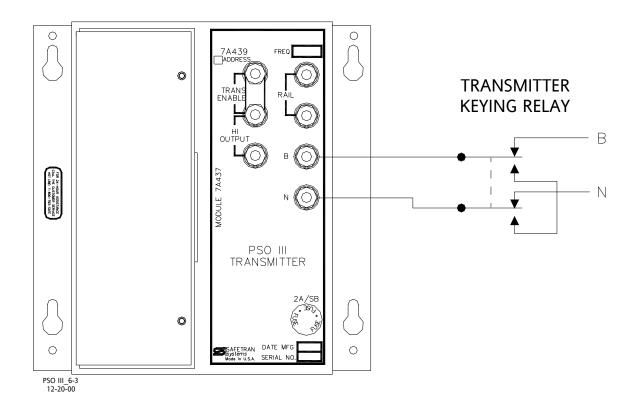
Figure 6-3 PSO III Transmitter Connections To Remote Keying Relay (Transmitter Shown Strapped For Continuous Low-Power Operation)
