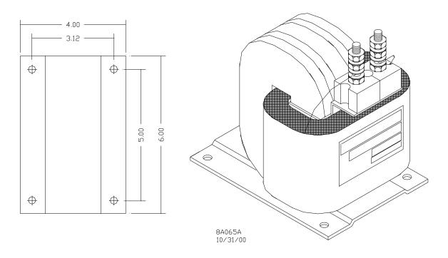
Figure 5-2 62648/8A065A Battery Choke With Mounting Dimensions
