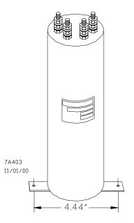
Figure 5-6 PSO Line Overlay Coupler, 7A403
