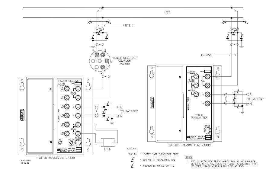
Figure 8-1 PSO III Installation With Tuned Receiver Coupler, 7A355A-f
