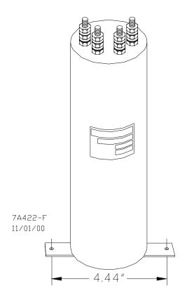
Figure 5-8 Tuned Insulated Joint Bypass Coupler, 7A422-f
