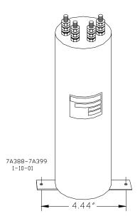
Figure 5-5 Typical of Line-To-Receiver Coupler, 7A388, and Transmitter Line-To-Rail Coupler, 7A399-f
