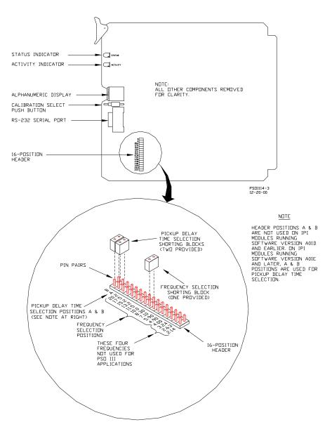
Figure 4-3 Jumper Positions On 16-Position Header
