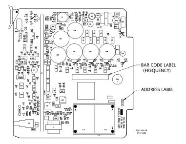
Figure 6-4 Location of Receiver Module Address and Frequency Labels
