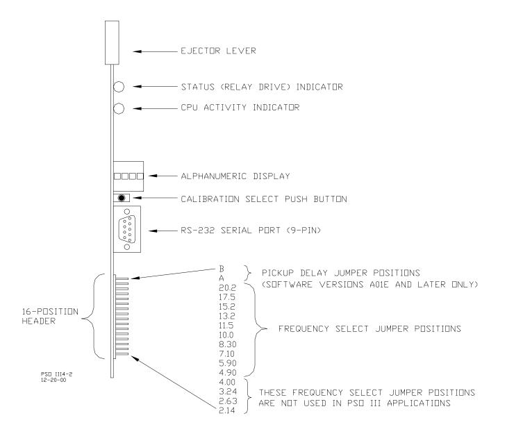
Figure 4-2 IPI Module Control And Indicator Locations
