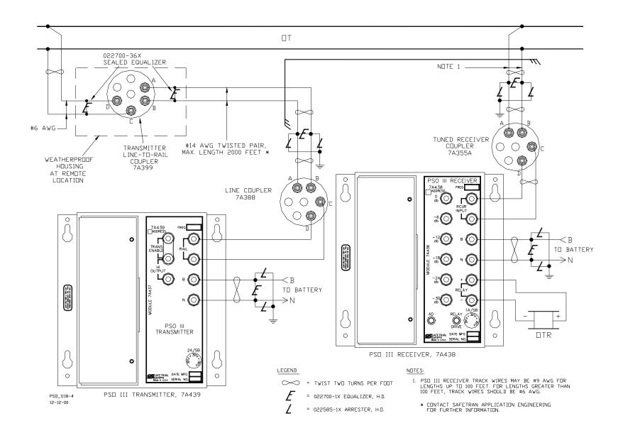
Figure 8-4 PSO III Installation With Transmitter Line-to-Rail Coupler, 7A399-f
