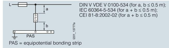
Recommended max. cable lengths for parallel connections
